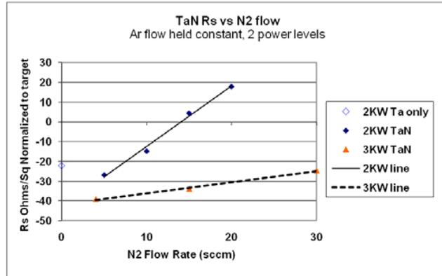
Figure 1: Graph of resultant Rs vs. N<sub>2</sub> flow rate for two power settings. Ar flow rate and dep time were held constant; the ratio of Ar to N<sub>2</sub> varied.
