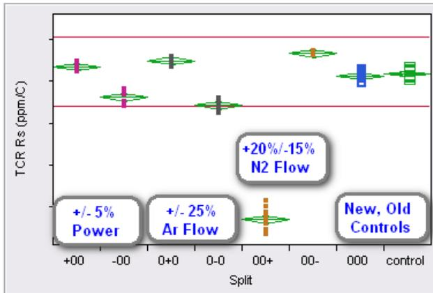
Figure 2: Graph of TCR to check range of major settings vs. TCR. Red lines define desired process region. 000=power, Ar flow, N<sub>2</sub> flow
