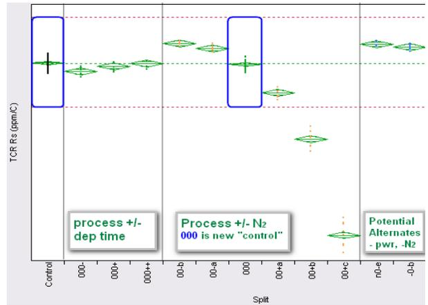
Figure 3: Graph of TCR to check effect of process variation from adjusting the controllable range of options inputs against process limits and target.
