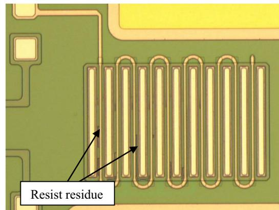
**Figure 1 Resist residue in the S/D electrodes**
