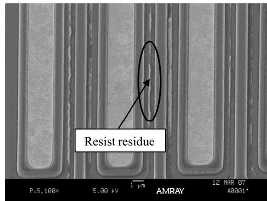
**Figure 2 Top view SEM image of resist residue**
