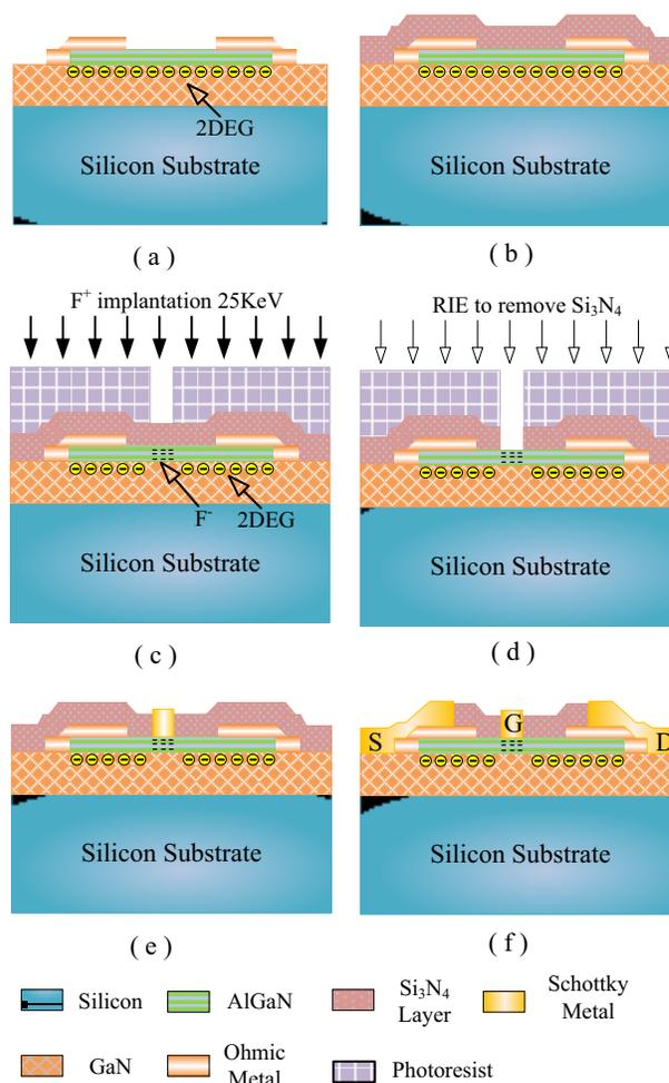
Fig. 1 Schematics showing the process flow of ion implanted E-mode HEMTs: (a) Active region and ohmic metal; (b) Si<sub>3</sub>N<sub>4</sub> layer deposition; (c) Gate area definition and fluorine ion implantation; (d) Si<sub>3</sub>N<sub>4</sub> layer etching; (e) Self-aligned gate metal deposition and lift-off; (f) Interconnection metal formation.
