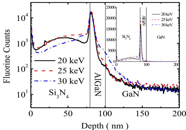
Fig. 5 Fluorine profiles measured by Secondary-Ion-Mass-Spectrometry (SIMS) of in Si<sub>3</sub>N<sub>4</sub>/AlGa<sub>N</sub>/GaN structure implanted with different energy ( 20 keV, solid; 25 keV, dash; 30 keV, dash and dot). The inset shows the profiles in linear scale.
