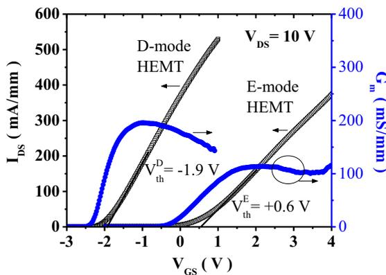
Fig. 2 Transfer characteristics of D-mode HEMTs and E-mode HEMTs with a gate length of 1 μm.
