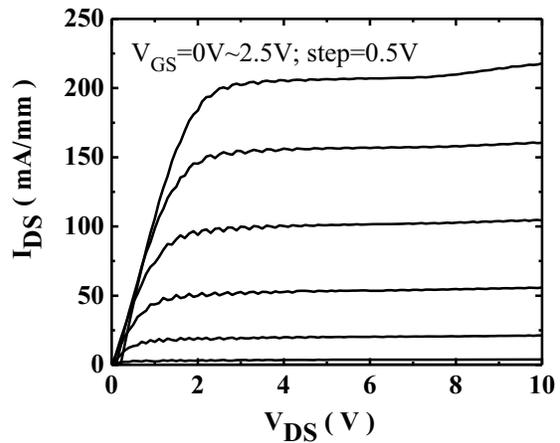
Fig. 3 DC output characteristics of E-mode HEMTs with a gate length of 1 μm. The gate-source spacing is 1 μm and the gate-drain spacing is 2 μm.
