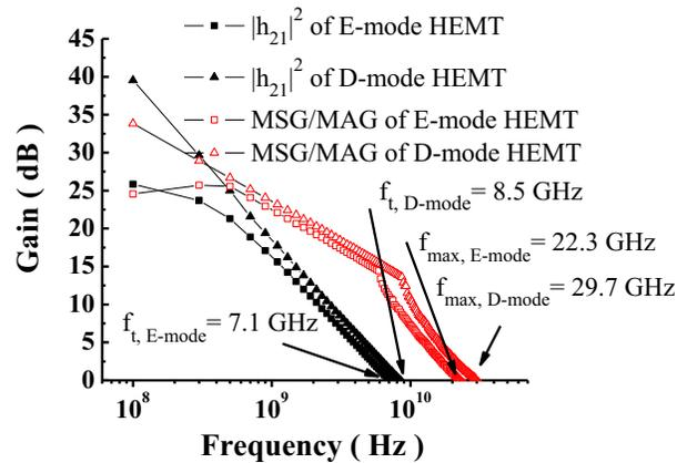
Fig. 4 Small-signal RF characteristics of D-mode and E-mode HEMT with a gate length of 1 μm, measured at bias  $V_{DS} = 12$  V,  $V_{GS} = -1.4$  V for D-mode HEMT and  $V_{DS} = 12$  V,  $V_{GS} = 3.0$  V for E-mode HEMT.
