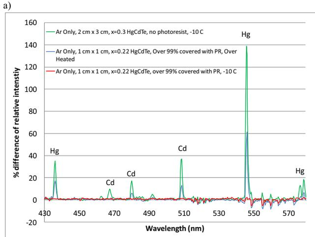
b) Figure 1.a) Optical emission spectra for Ar only processed HgCdTe Test samples b ) intensity difference between samples with HgCdTe, and photoresist normalized on an Ar only processed Si wafer. Ar only plasma used to test low etch rates.
