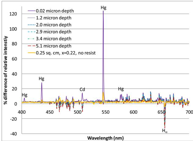
Figure 3. Intensity difference between samples with HgCdTe, photoresist and plain Si wafer. Xe H<sub>2</sub> 4:1, 2 cm x 2 cm, x=0.22 HgCdTe, over 99% covered with PR, Via Pattern, -40 C temperature. Xe H<sub>2</sub> 4:1, ~0.25 cm<sup>2</sup>, x=0.22 HgCdTe, no PR, -10 C temperature, ~0.5 etch depth.
