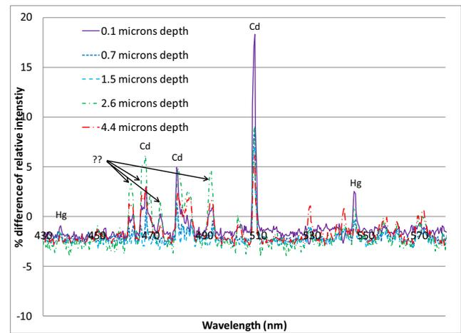
Figure 2. Intensity difference between samples with HgCdTe, photoresist and plain Si wafer. Xe only,  $1 \text{ cm} \times 0.5 \text{ cm}$ ,  $x=0.7 \text{ HgCdTe}$ ,  $\sim 1\%$  covered with PR, Mesa Pattern,  $-10 \text{ }^\circ\text{C}$  temperature.
