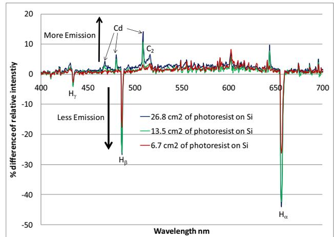
Figure 4. Intensity difference between samples with photoresist and samples without photoresist. No intention HgCdTe used. Ar / H<sub>2</sub> 4:1 gas ratio
