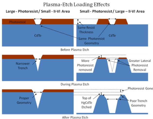
Figure 5. Example of macro-loading effect as measured in reference 17.
