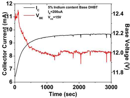
**Figure 3. The measured collector current and base voltage during constant base current stressing ( $I_B = 200 \mu\text{A}$ )**
