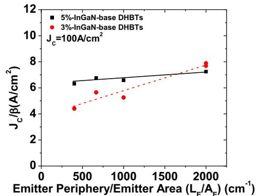
**Figure 2.**  $J_C/\beta$  plotted against the emitter perimeter-to-area ratio ( $L_E/A_E$ ) for  $J_C = 100 \text{ A/cm}^2$  for 3%-InGaN-base and 5%-InGaN-base DHBTs.
