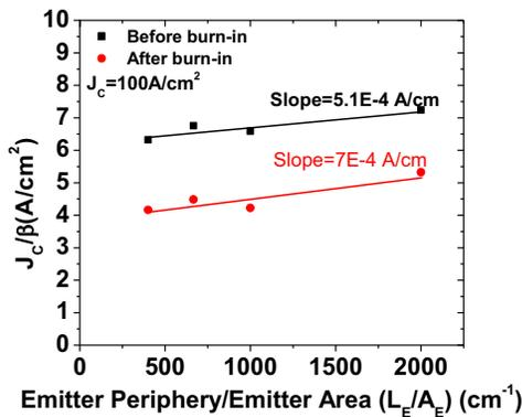
**Figure 4  $J_C/\beta$  plotted against the emitter perimeter-to-area ratio ( $L_E/A_E$ ) before and after burn-in.**
