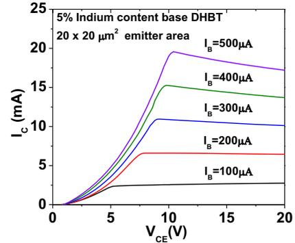
**Figure 1.** Common-emitter characteristics of a fabricated GaN/In<sub>0.05</sub>Ga<sub>0.95</sub>N DHBT with  $A_E = 20 \times 20 \mu\text{m}^2$
