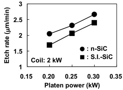
Fig. 6. Platen power dependence of etch rate for n-SiC and S.I.-SiC. The via-hole diameter is 150  $\mu\text{m}$ .
