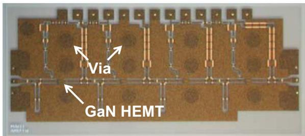
Fig.9. Photomicrograph of the fabricated MMIC LNA with GCPW. Its size is  $3.0 \times 1.4 \text{ mm}^2$ .
