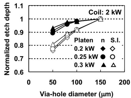
Fig. 7. Via-hole diameter dependence of normalized etch depth in both SiC substrates.
