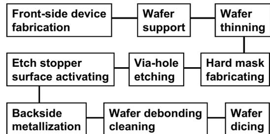
Fig. 3. Flow chart for GaN HEMT MMIC backside process.
