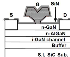
Fig. 1. Cross-sectional view of millimeter-wave GaN HEMT.
