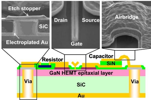
Fig. 2. Schematic millimeter-wave GaN HEMT MMICs.
