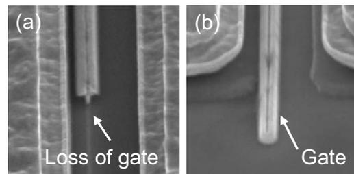
Fig. 8. SEM images of 0.1- $\mu\text{m}$  gate-length GaN HEMT with 50-nm-thick SiN passivation layer after dicing: (a) without polymer and (b) with polymer.
