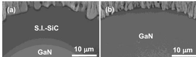
Fig. 5. SEM image of via-hole bottom for GaN HEMT/S.I.-SiC wafer.
