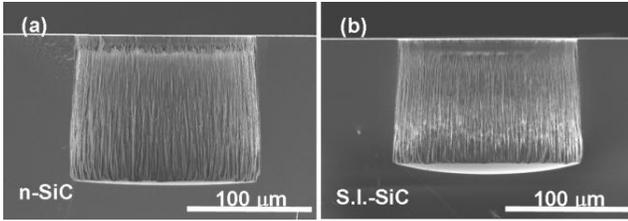
Fig. 4. Cross-sectional SEM images of 150  $\mu\text{m}$ -diameter via-holes etched at the coil/platen powers of 2/0.3 kW: (a) n-SiC and (b) S.I.-SiC.
