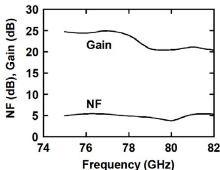
Fig. 10. Measured NF and gain of LNA ( $V_{ds}=10\text{V}$ )
