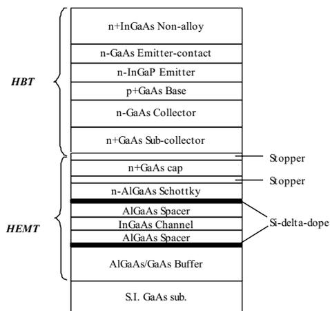
Fig.1 Schematic diagram of BiHEMT structure
