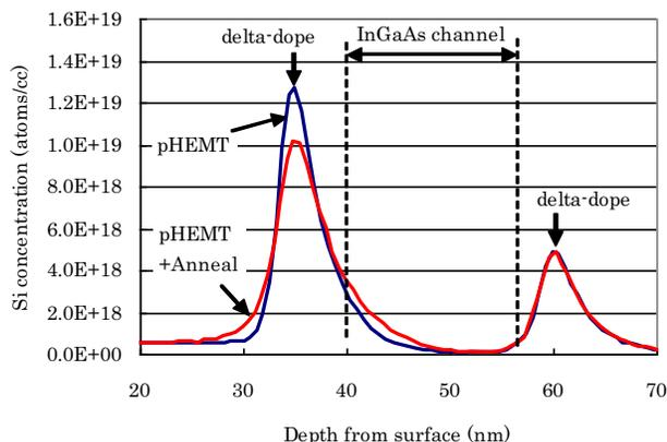
Fig.5 SIMS profile of Si in the pHEMT before and after the annealing
