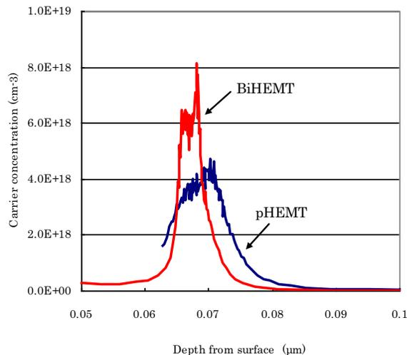
Fig.3 C-V profiles of pHEMT in BiHEMT and Simple pHEMT
