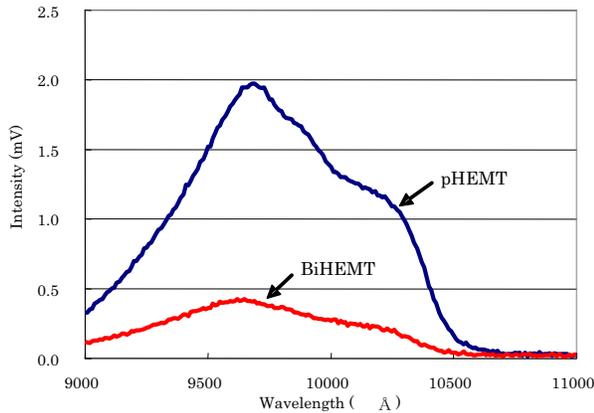
Fig.2 PL profiles of pHEMT in BiHEMT and simple pHEMT
