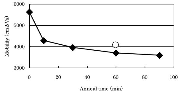
Fig.4 Degradation of mobility by annealing effect
