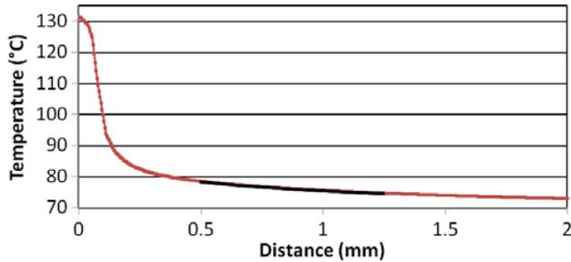
Figure 2: Red line: Modeled temperature from the center of the heat source along the top of the wafer, based on the geometry of Fig. 1 and with 20 kW/m<sup>2</sup>/K wafer-chuck resistance. Black line: A fit of  $dT/dr = A/r$  to the portion of the profile for which  $500 \mu\text{m} < r < 1250 \mu\text{m}$ , where  $r$  = distance from the center of the heat source, where  $A$  is a constant. This fit deviates from the model data by less than 0.1 °C within this region.
