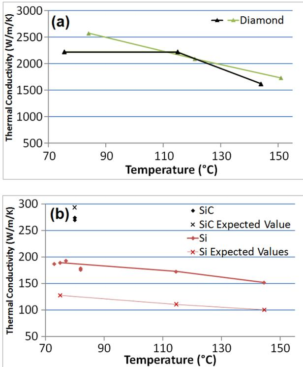
Figure 4: Temperature dependent thermal conductivity data for the wafers tested (diamond, Si and SiC) and compared to expectations for Si and SiC. The diamond data (a) is from two test structures on the same wafer. Multiple data sets exist for each material because of testing under different conditions, although experimental data connected by lines represent data collected under the same conditions except for baseplate temperature.
