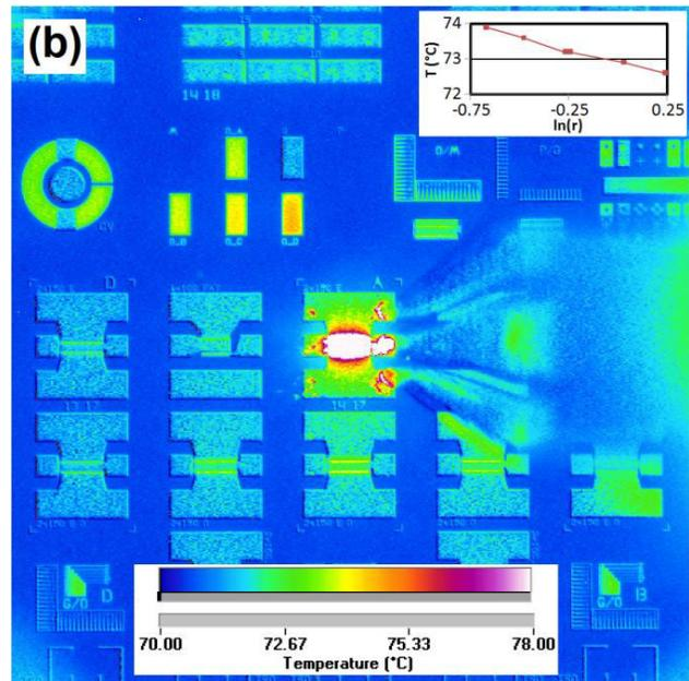
Figure 3: An IR emissivity map (a) and corresponding temperature map (b). Both measure 2400  $\mu\text{m}$  to a side. The arrows show the features on which acceptable data were collected. The emissivity map clearly shows the probes used to power the device; no data can be collected there. The inset shows the plotted temperature vs. natural log of the distance (measured in mm) from the center of the heat source, plotted in this way to make the relationship linear.
