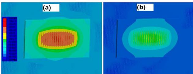
**Figure 2:** Temperature distribution in AlGaIn/GaN HEMT (18 fingers power bar) for a dissipated power level of 30W obtained from 3-D finite element simulation for (a) device brazed onto CuW base plate, and (b) onto diamond composite base plate.
