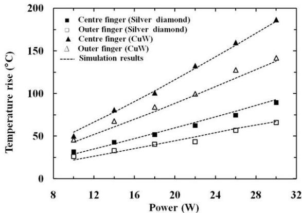
**Figure 1:** Peak temperature rise in the centre finger of AlGaIn/GaN HEMTs devices (18 fingers power bar) brazed to silver diamond composite and CuW base plates as a function of the dissipated power, obtained by Raman thermography. 3-D finite element thermal modeling results are shown for comparison.
