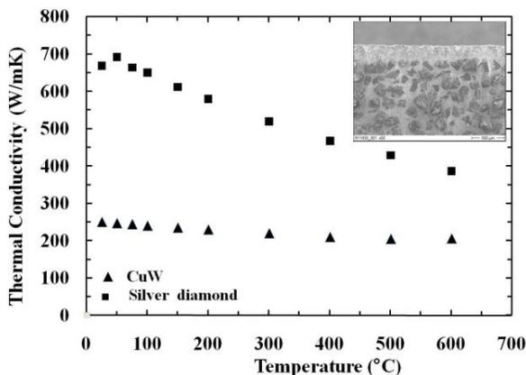
**Figure 3:** Thermal conductivity as a function of temperature for silver diamond composite and CuW materials. In the inset a SIM image of silver diamond is shown.
