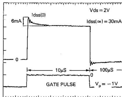
Figure 1. Shown is a drain current transient effect due to an incident gate pulse.
