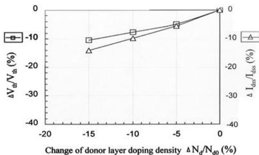
Figure 2. Donor compensation effects due to trapping effects results in a change in donor layer density.
