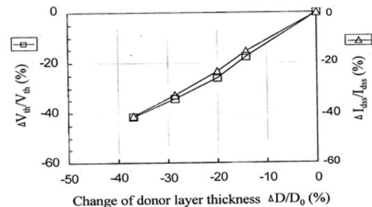
Figure 3. A decrease in saturation current which may result from gate degradation effects is shown in the above figure.
