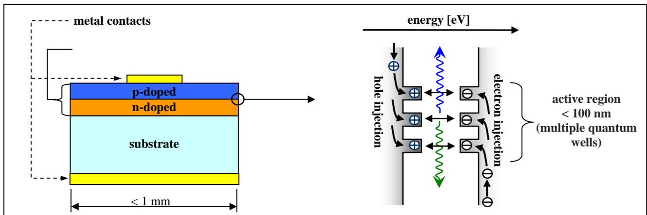
Figure 1: LED-functional principle: schematic cross view (left) and energy band diagram (right)
