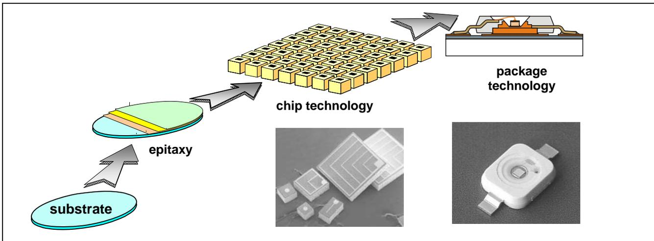
Figure 2: LED process chain
