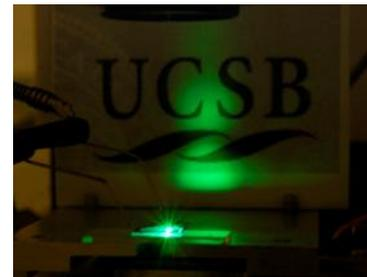
Figure 4: Far field image of the semipolar (20 $\bar{2}$ 1) laser diode demonstrated at UCSB.
