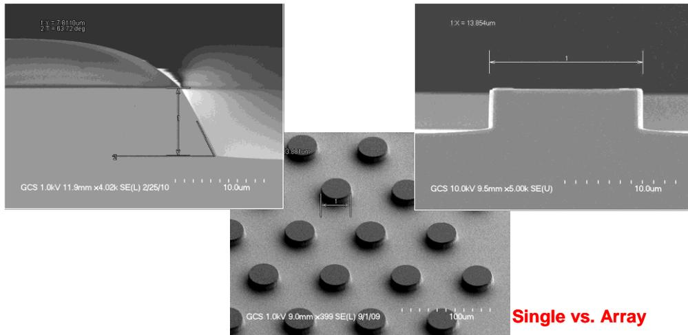
Figure 3. Different dry etch recipes to satisfy different “VCSEL” design requirements for vertical vs. sloped mesa sidewalls and single element vs. arrayed device.
