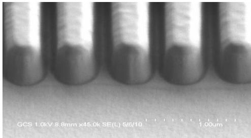
Figure 1. Laser gratings with 0.06um spacings.
