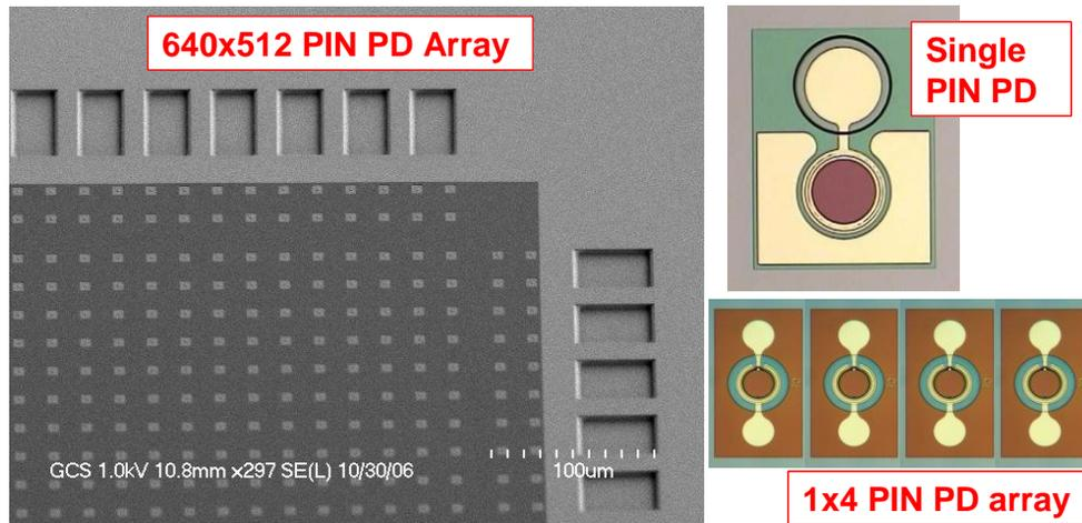
Figure 5. InGaAs PIN PD process - from simple discrete device to complicated large format imaging array.
