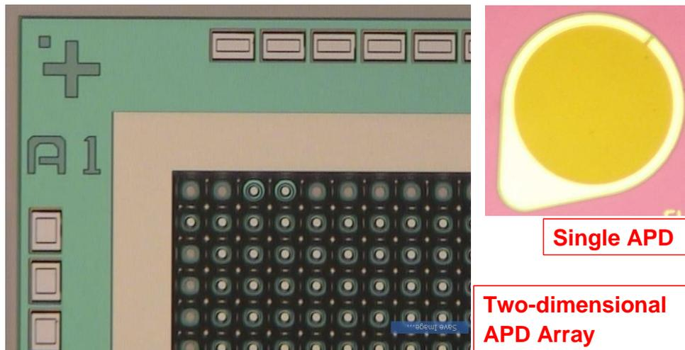
Figure 6. APD process module can produce discrete APD as well as large format two-dimensional APD array.
