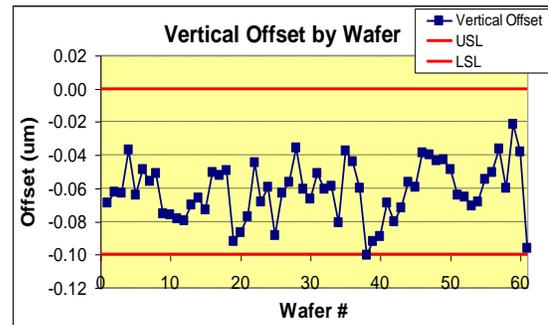
Figure 2. Laser vertical offset SPC.
