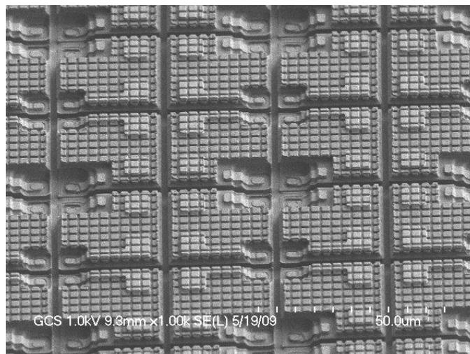
Figure 4. Opto device with 10-15um sloped or vertical sidewalls for continuous interconnect metal step coverage.
