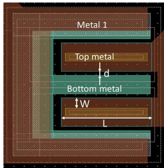
Fig.1. Interdigitated Layout design of tilted-charged LED
