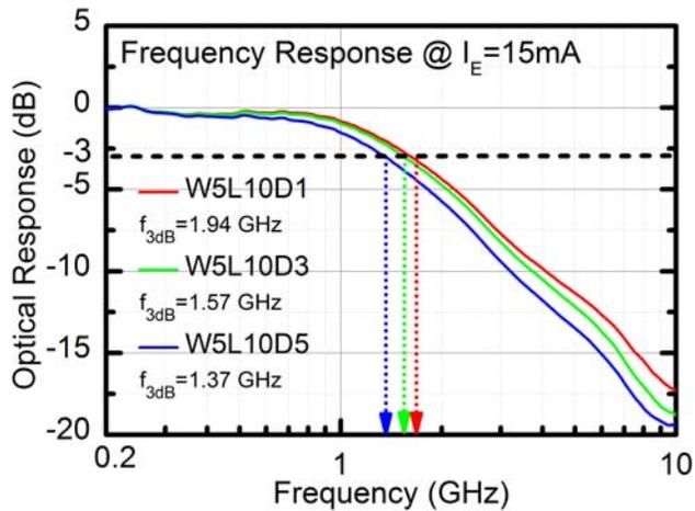
Fig. 4. The frequency response of devices with  $d=1, 3,$  and  $5\mu\text{m}$ .
