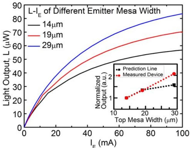
Fig. 2. The L-I<sub>E</sub> curve of tilted-charge LED with different top mesa, the inset shows the normalized light output intensity versus the mesa width
