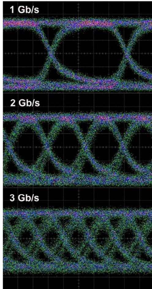
Fig. 5. The eye diagrams of tilted-charge LED operating at  $1, 2,$  and  $3\text{Gb/s}$ , respectively.
