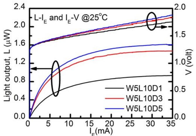
Fig. 3. The  $L-I_E$  and  $I_E-V$  characteristic. Note that the increase in  $d$  gives higher resistance as the slope of I-V curves goes down.
