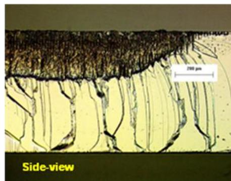
Figure 4, Side-view of a GaAs substrate with interrupted first laser dicing pass, made visible by breaking of the sample.
