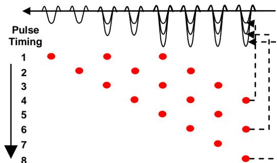
Figure 3, Schematic of the multiple beam process during one laser pass
