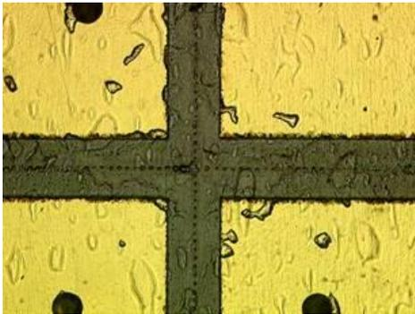
Figure 7, Example of a laser diced 100um full Au wafer with a dicing width <math><17\mu\text{m}</math> and effective dicing speed >math>>75\text{mm/s}</math>
