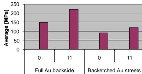
Figure 8, 4-point Die strength comparison of GaAs substrates with full Au metal backside and with back-etched streets
