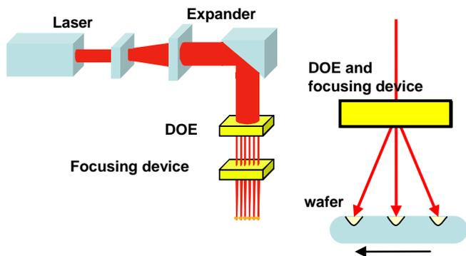
Figure 2, Concept of the multi beam laser dicing technology showing an overview (left) and shown in detail with substrate (right)
