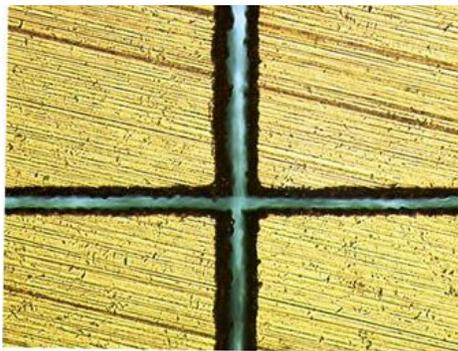
Figure 6, Example of a laser diced 100um full Cu wafer with a dicing width <24um and effective dicing speed>60mm/s
