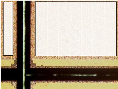
Figure 5, Example of a laser diced CuW LED wafer of 215um thickness with Au back metal
