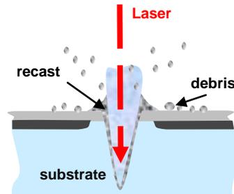
Figure 1, Principle of ablation laser dicing
