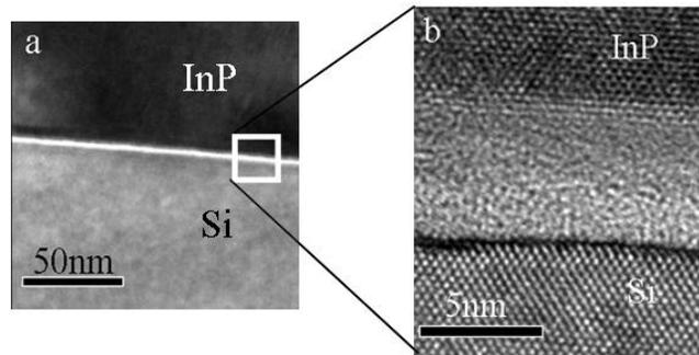
Figure 2. Cross section TEM images of InP/Si bonding interface after annealing at 300°C for 120hrs, a and b stand for TEM and HRTEM pictures, respectively.
