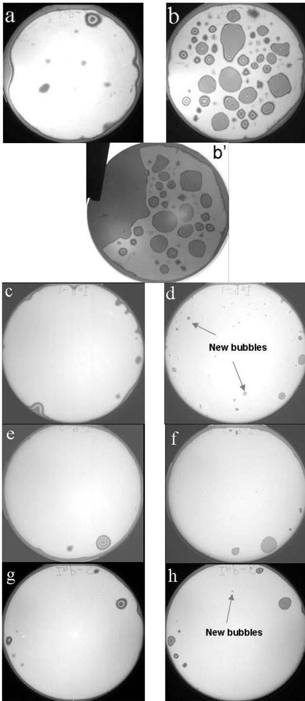
Figure 1. Infrared images of InP/Si bonded pairs, a, c, e, g, before annealing for 0s, 20s, 40s, 60s plasma exposure, respectively. b, d, f, h corresponding to a, c, e, g after annealing at 300°C for 120hrs. b' with a blade from b.
