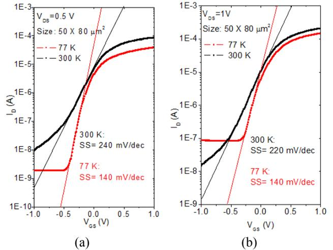
Fig. 6. Temperature dependent  $I_D$ - $V_{GS}$  characteristics of a  $\text{In}_{0.53}\text{Ga}_{0.47}\text{As}/\text{InAs}/\text{InP}$  TFET. (a) At  $V_{ds} = 0.5$  V, the minimum point subthreshold swing  $SS_{\min}$  decreased from 240 mV/dec at 300 K to 140 mV/dec at 77 K; (b) at  $V_{DS} = 1$  V  $SS_{\min}$  decreased from 220 mV/dec at 300 K to 140 mV/dec at 77 K.
