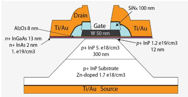
Fig. 1. Cross section of a vertical  $\text{In}_{0.53}\text{Ga}_{0.47}\text{As}/\text{InAs}/\text{InP}$  TFET fabricated using a gate first self-aligned process.
