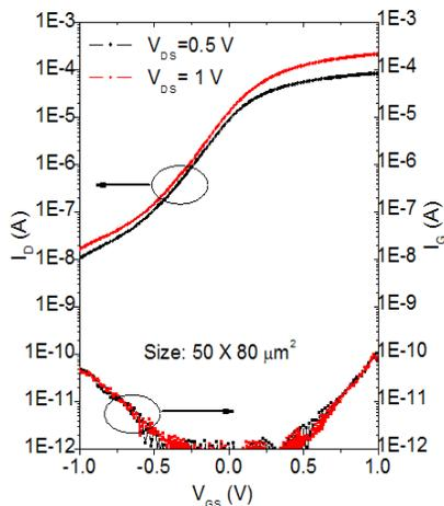
Fig. 5. Measured transfer curves and gate leakage current on a self-aligned  $\text{In}_{0.53}\text{Ga}_{0.47}\text{As}/\text{InAs}/\text{InP}$  VTFET at 300 K.
