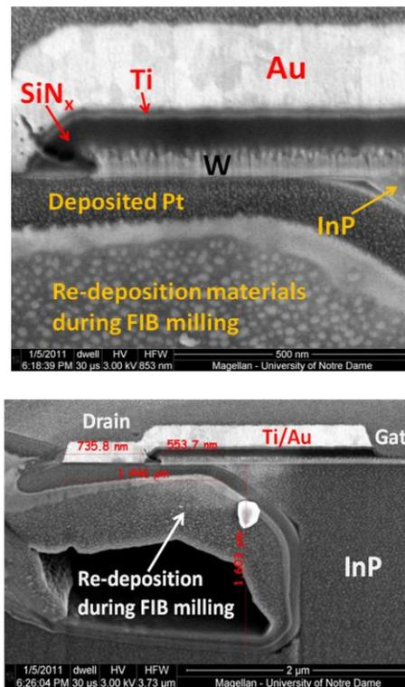
Fig. 3. FIB/SEM cross sections of a fabricated vertical  $\text{In}_{0.53}\text{Ga}_{0.47}\text{As}/\text{InAs}/\text{InP}$  TFET: (upper) featuring  $\text{SiN}_x$  sidewall and  $\text{InP}$  undercut etch, and (lower) a lower-magnification view of the self-aligned drain contact and device structure after etching in  $\text{HCl}:\text{H}_3\text{PO}_4$  (1:3).
