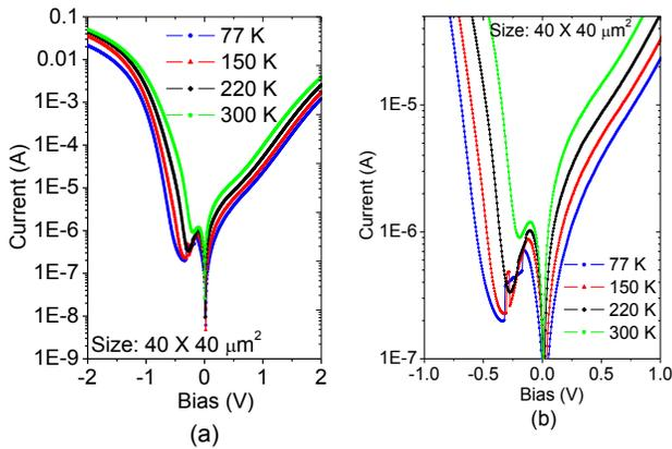
Fig. 7. (a) Representative current-voltage characteristics of the  $p+\text{InP}/n+\text{InAs}/n+\text{In}_{0.53}\text{Ga}_{0.47}\text{As}$  tunnel junction for temperatures ranging from 77 to 300 K. (b) Expanded view of the temperature dependence in the current range about the NDR.
