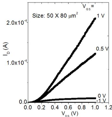
Fig. 4.  $I_D$  versus  $V_{DS}$  for gate voltage  $V_{GS}$  stepped from -1 to 1 V of a self-aligned  $\text{In}_{0.53}\text{Ga}_{0.47}\text{As}/\text{InAs}/\text{InP}$  VTFET at 300 K.
