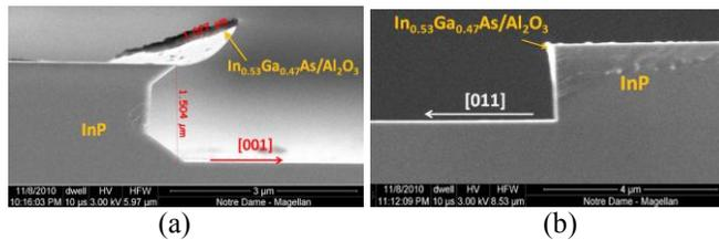
Fig. 2. Cross section of  $\text{InP}$  profile after etching with mask aligned perpendicular (a) to  $[001]$  showing significant  $\text{InP}$  undercut and (b) to  $[011]$  showing negligible  $\text{InP}$  undercut or etch.
