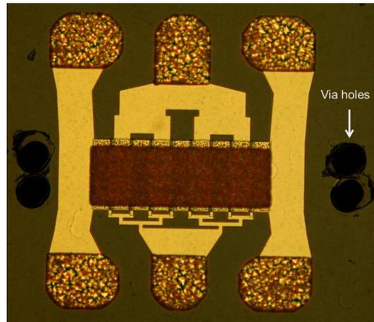
Figure 4. An eight finger device prior to via metallization.
