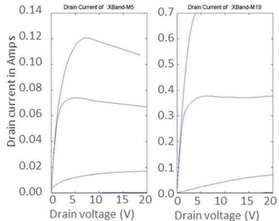
Figure 5. The IV characteristics of a two (left) and an eight (right) finger HEMT device on diamond.
