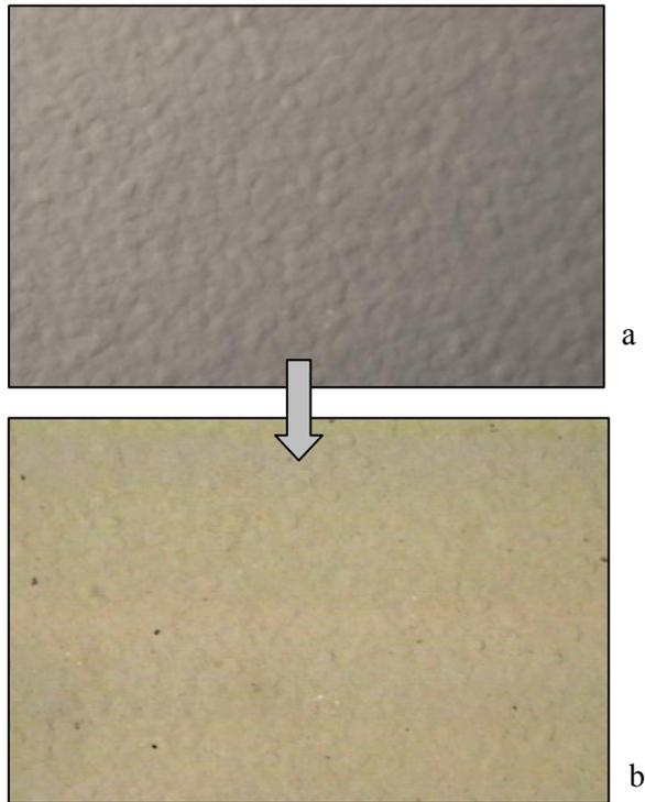
Figure 1. Nomarski micrographs (20x lens) of epi surface before (a) and after (b) transfer to diamond.
