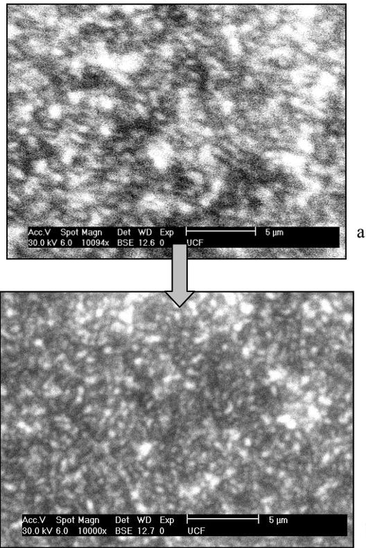
Figure 3. Show the CL map of the GaN epi surface before (a) and after (b) transfer to a diamond substrate.
