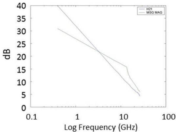
Figure 6. The small signal frequency response of an eight finger HEMT on diamond.
