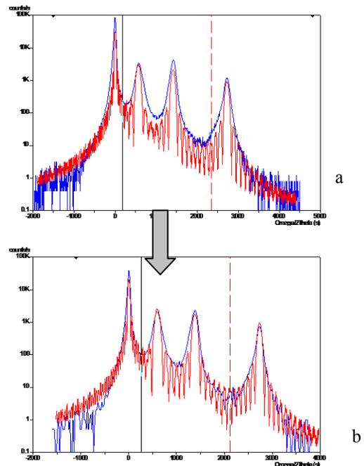
Figure 2. Experimental (blue) and calculated (red)  $\omega$ -2 $\theta$  rocking curves for (0002) reflection, measured in the vicinity of GaN/AlN peaks before (a) and after transfer to diamond.
