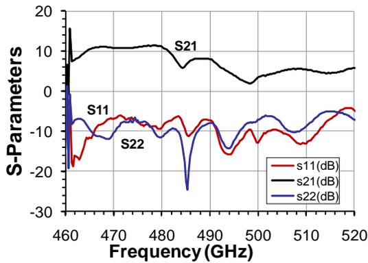
Fig. 2. Measured S-Parameters of 0.48 THz amplifier [6].
