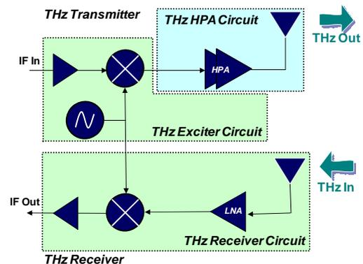
Fig. 1. Conceptual block diagram of the THz Electronics transceiver.
