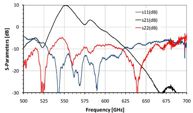
Fig. 3. Measured S-Parameters of cascode amplifier. A peak measured gain of 10 dB has been measured at 550 GHz was measured in package. A micrograph of the [7].
