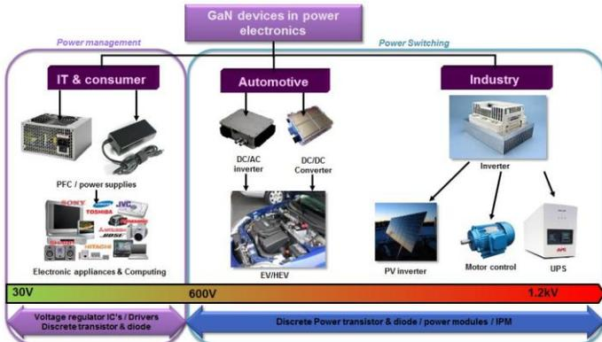
Figure 1: Fields of applications for GaN power devices
