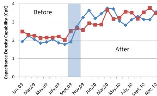
**Figure 6.** Capacitance density capability before and after the implementation of the optimized chamber clean. Shaded region shows implementation period.
