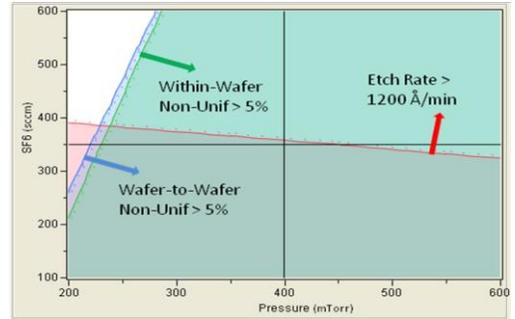
**Figure 2.** Chamber clean etch rate and uniformity results modeled with respect to pressure and SF<sub>6</sub> flow rate. The N<sub>2</sub>O flow rate is held constant at 350 sccm.
