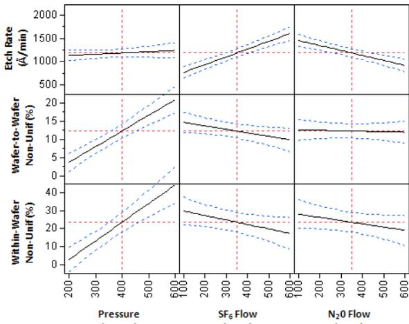
**Figure 1.** Chamber clean etch rate and non-uniformity results modeled with respect to pressure, SF<sub>6</sub> flow rate, and N<sub>2</sub>O flow rate.
