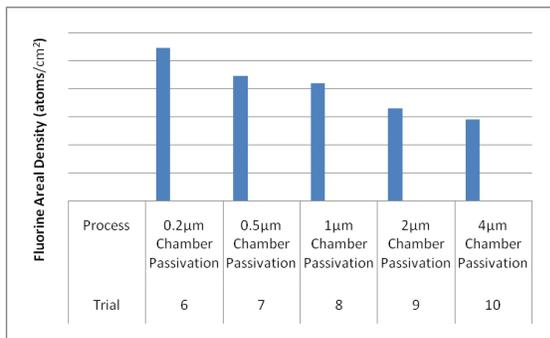
Figure 9. Fluorine concentrations in post chamber clean  $\text{SiN}_x$  films with respect to post chamber clean passivation thickness.
