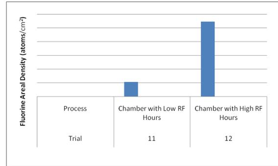
Figure 10. Fluorine concentrations in post chamber clean  $\text{SiN}_x$  films with respect to chamber RF hours.
