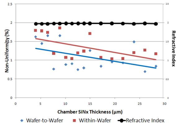
**Figure 3.** Refractive index and non-uniformity vs. chamber SiN<sub>x</sub> thickness.
