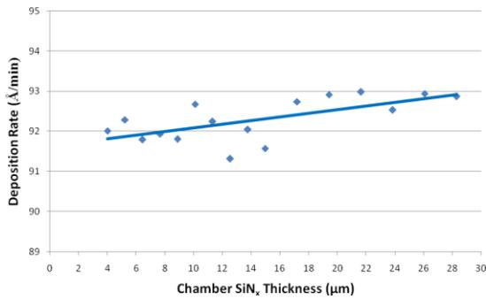
**Figure 4.** SiN<sub>x</sub> deposition rate vs. chamber SiN<sub>x</sub> thickness.
