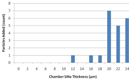
**Figure 5.** Particles added vs. chamber SiN<sub>x</sub> thickness.
