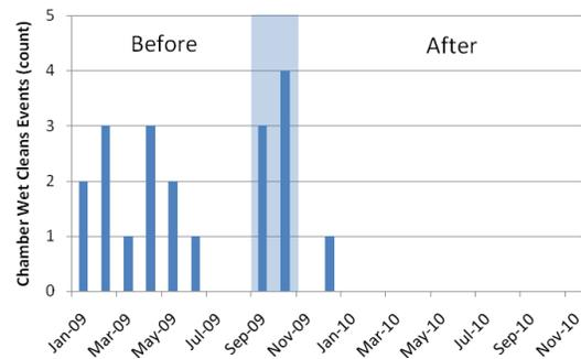
**Figure 7.** Chamber wet clean events per month before and following the implementation of the optimized SF<sub>6</sub>/N<sub>2</sub>O clean. Shaded region shows implementation period.
