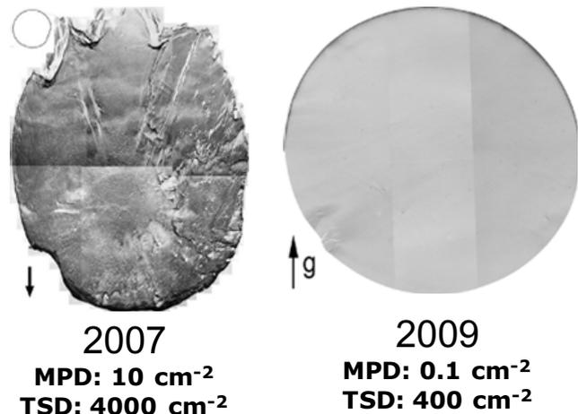
Figure 1. Reflection x-ray topography (XRT) images of 76 mm diameter n+ 4H SiC crystals. Left: Original PVT Process; Right: Improved PVT Process.
