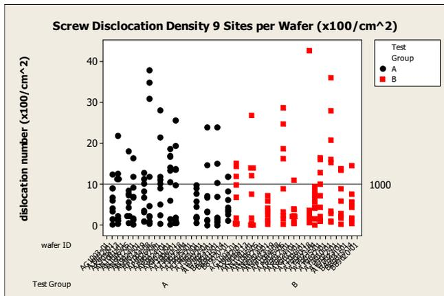
Figure 3. Measurements of screw dislocation density on wafers from over 25 crystals of n+ 4H SiC. Data was collected by x-ray topography and counting was performed at nine sites on each wafer. Each column of points represents the nine measurements on each wafer. The groups represent two sampling points of manufactured product over the period from midyear 2009 to midyear 2010.
