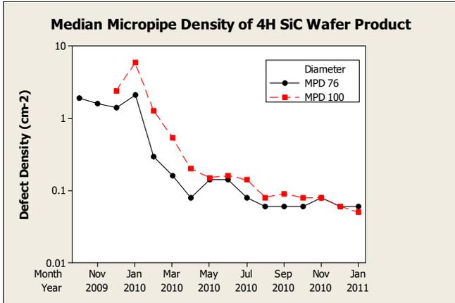
Figure 2. Median micropipe defect density of conducting 4H SiC wafers of both 76 mm and 100 mm diameter manufactured over five quarters.
