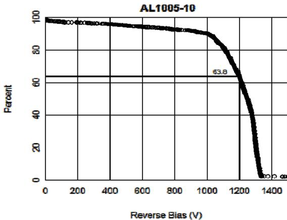
Figure 5. Distribution of diode blocking voltages measured on 76 mm diameter 4H SiC epiwafer, 8.3 um thick, average doping 1.6E16/cm<sup>3</sup>.
