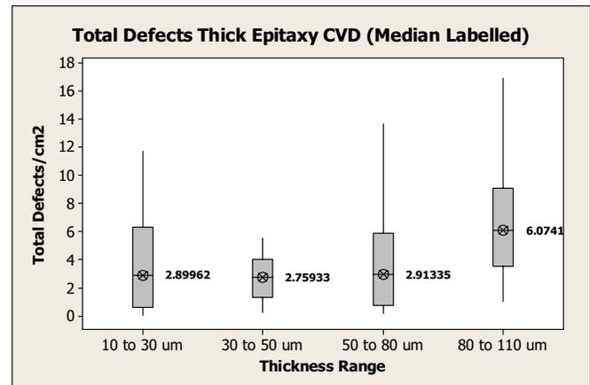
Figure 7. Distribution of total defects (substrate and epitaxy added defect, inclusive) in 76 mm diameter research 4H SiC epiwafers for high voltage applications measured by laser light scattering spectrometry.
