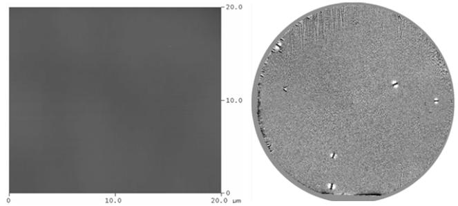
Figure 6. AFM image of the wafer center (left) and whole wafer laser light scattering topograph image (right) of a 76mm diameter 4H SiC wafer with 100 um epitaxy. The AFM image is featureless and shows average roughness is 0.7 nm. The measured total defect density is 1.9/cm<sup>2</sup>.
