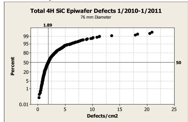
Figure 4. Distribution of total defects (substrate and epitaxy added defect, inclusive) for 76 mm diameter production 4H SiC epiwafers measured by laser light scattering spectrometry. Thickness of the epitaxial films typically in the range of 5-15 um.
