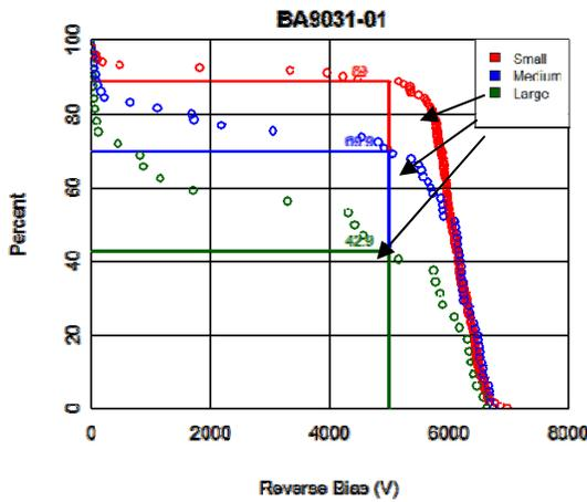
Figure 8. Distribution of diode blocking voltages measured on 76 mm diameter 4H SiC epiwafer, averaging 52  $\mu$ m thick, with average doping  $8.5E14/\text{cm}^3$ .
