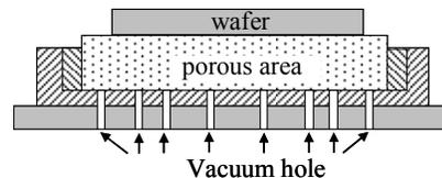
Figure 9 wafer chuck table cross section
