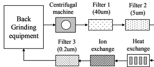
Fig.5 water recycling system
