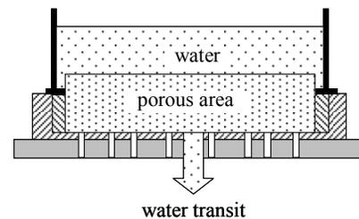
Figure10. Evaluation method of chucking power
