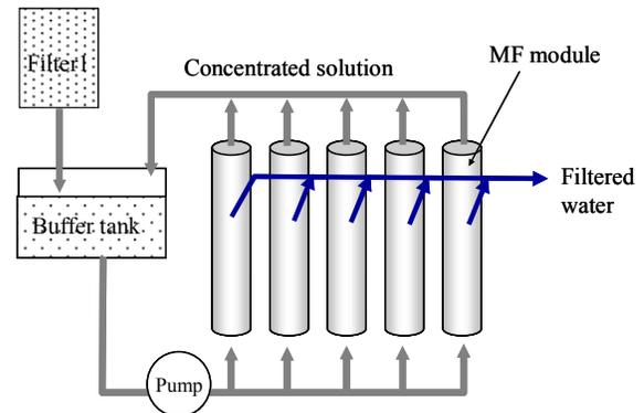
Fig.7 MF membrane system
