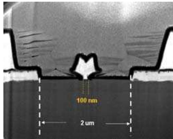
Figure 1. The cross-section picture of the 0.1 $\mu$ m GaAs pHEMT device.
