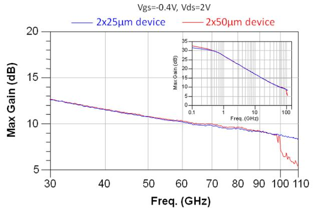
Figure 4. The maximum gain performance is measured by  $110\text{GHz}$  S-parameters system. The MSG of both  $2\times 25\mu\text{m}$  and  $2\times 50\mu\text{m}$  transistors could be maintained about  $8\text{dB}$  at  $90\text{GHz}$ .
