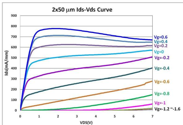
Figure 3. The IV curve of PP10. We can see the knee voltage below a drain voltage of  $1\text{V}$  and superior large voltage swing area for the RF signal.
