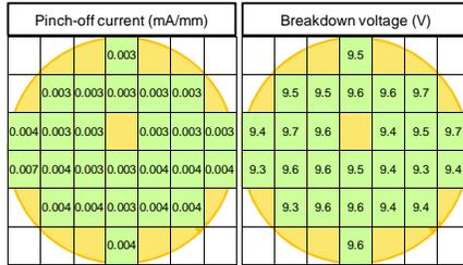
Figure 7. The gate yield is determined by gate leakage, pinch-off, and breakdown performance of the 25x75um device.
