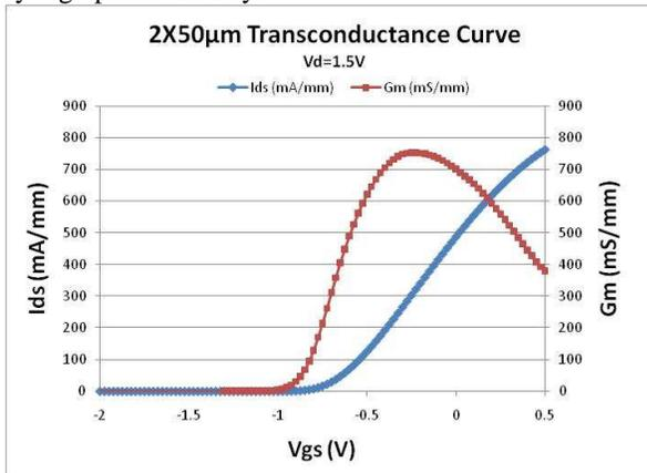
Figure 2. The transconductance curve of PP10. A high current and transconductance behavior are observed.
