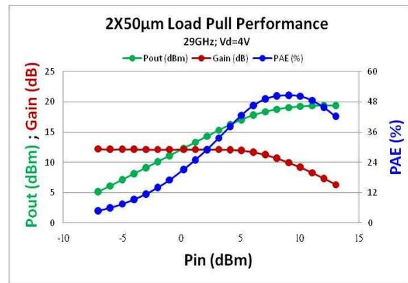
Figure 5.  $850\text{mW/mm}$  saturated power density could be reached under  $29\text{GHz}$  load pull system, the device is operated at drain bias of  $4\text{V}$ .
