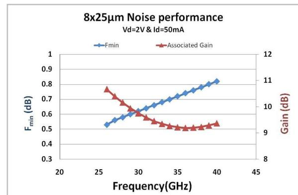
Figure 6. The  $26\text{-}40\text{GHz}$  noise performance of PP10 that taken at  $V_{ds}=2\text{V}$  and  $50\text{mA/mm}$ .
