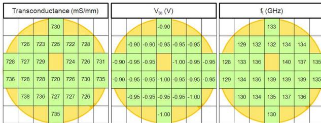
Figure 8. The wafer maps of the key parameters of 2x75um device show high uniformity.
