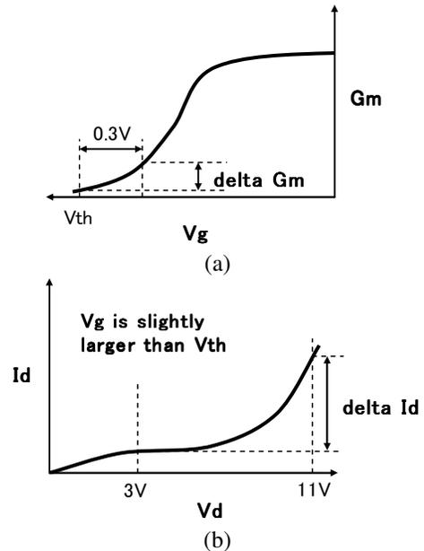
Fig. 5 Definitions of (a) delta Gm and (b) delta Id. (a) quantifies the electron flow near the buffer and (b) quantifies the leakage current in buffer.
