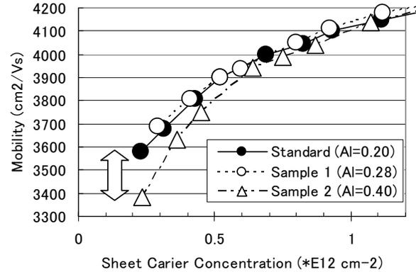
Fig. 7 Results of Hall measurement. Hall measurement and wet etching were repeated to know depth dependence of mobility.
