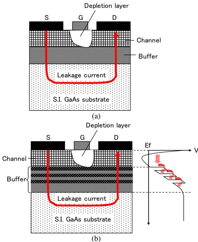
Fig. 9 Schematic image of (a) leakage current flow through buffer layer and (b) the leakage current flow of multiple buffer.
