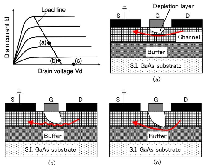
Fig. 1 Typical I-V characteristics of FET and schematic image of electron flow in each  $V_g$  condition. (a) and (b) are operating points of class A and B, respectively. At (c), depletion layer reached to buffer layer.
