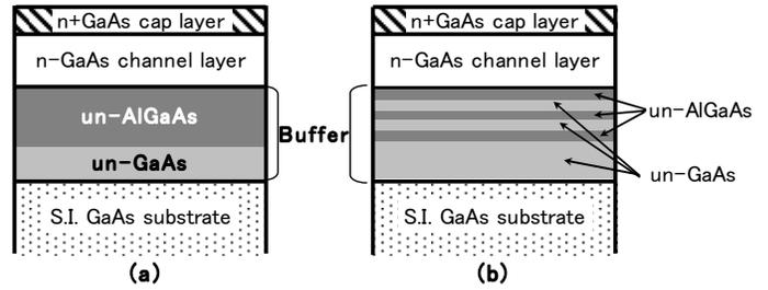
Fig. 4 MESFET epitaxial structure with (a) single AlGaAs buffer, (b) multiple AlGaAs/GaAs buffer.
