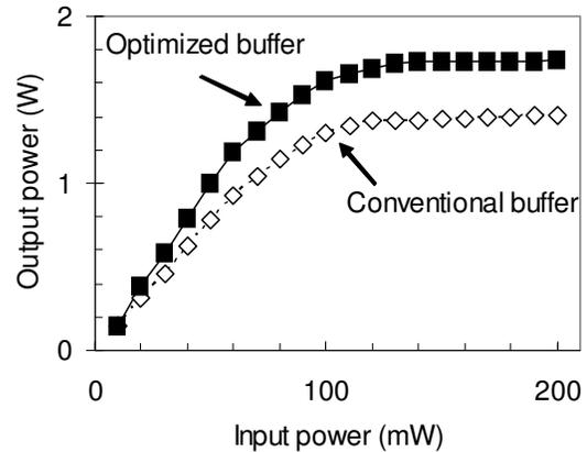
Fig. 10 Comparison of MESFET output power between conventional and optimized buffer.
