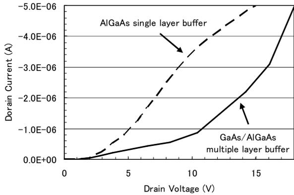
Fig. 8 Comparison of leakage current between AlGaAs single layer and i-GaAs/i-AlGaAs multiple layer buffer.
