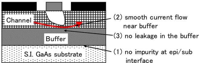
Fig. 3 The important features to improve high voltage performance.
