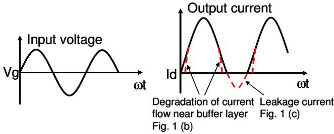
Fig. 2 Schematic images of input and output. Broken lines in output current show the noise elements.
