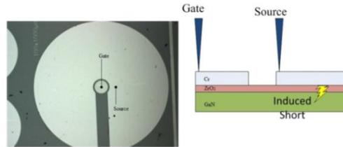
Figure 1: The top view of a typical  $100 \times 1000 \mu\text{m}$  MOSCAP, and an illustrated cross section.
