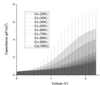
Figure 2: Spreading effects lower the effective capacitance as the measurement frequency increased.
