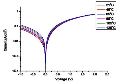
Figure 6: Variations in temperature had little effect on the thinner gate oxide consistent with direct tunneling.
