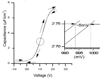
Figure 3: A CV sweep of the thinner at 20 KHz revealed the MOSCAP displayed little hysteresis.
