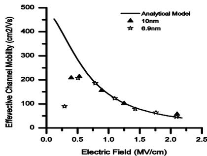
Figure 4: The effective electron mobility through the GaN is consistent for both the 6.9nm and 10 nm oxides.
