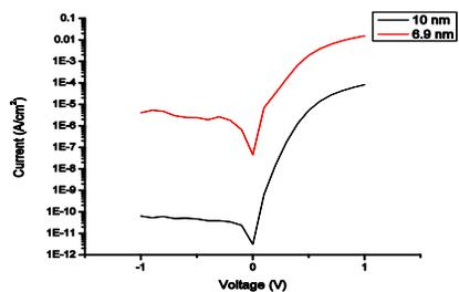
Figure 5: The gate oxides display near ideal tunneling current that scales appropriately with oxide thickness.
