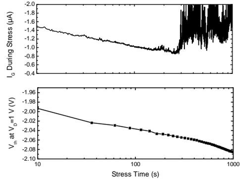
Fig. 2: variation of the (top) gate current and (bottom) threshold voltage for a HEMT submitted to constant voltage stress ( $V_G=-30$  V,  $V_D=V_S=0$  V)
