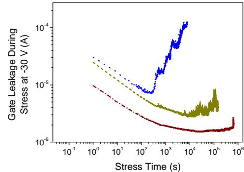
Fig. 8: variation of gate current for three HEMTs submitted to constant voltage stress ( $V_G=-30$  V,  $V_D=V_S=0$  V). The three HEMTs (located on the same wafer) have identical structures, and different initial leakage current levels (due to different initial defectiveness levels). Time to breakdown significantly depends on initial leakage level (this was verified on a larger set of samples, as reported in the text)
