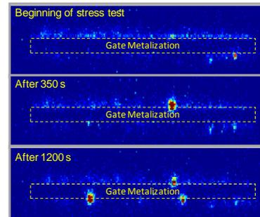
Fig. 4: spatially-resolved EL pattern recorded at increasing stress times on a HEMT submitted to constant voltage stress ( $V_G=-30$  V,  $V_D=V_S=0$  V, same device as in Fig. 2)
