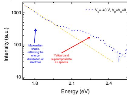
Fig. 5: EL spectrum of a reverse-biased HEMT, collected at  $V_G=-40$  V,  $V_D=V_S=0$  V
