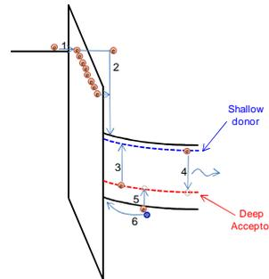
Fig. 6: schematic description of the model used to explain the recoverable degradation of AlGaIn/GaN HEMTs submitted to constant-voltage reverse-bias stress
