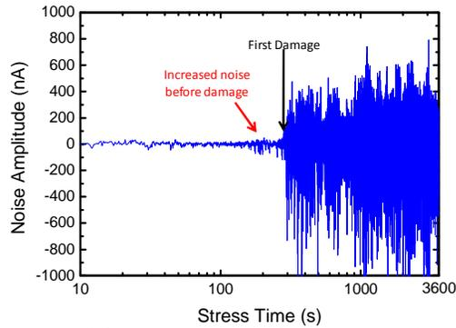
Fig. 3: variation of the noise superimposed to gate current, for a HEMT submitted to constant voltage stress ( $V_G=-30$  V,  $V_D=V_S=0$  V, same device as in Fig. 2)
