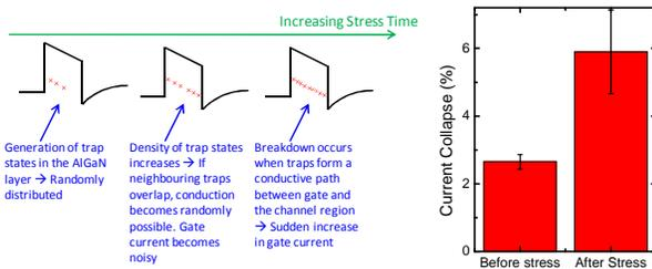
Fig. 7: (left) schematic description of the model used to explain permanent degradation of AlGaIn/GaN HEMTs submitted to constant-voltage reverse-bias stress. (right) results of current collapse measurements carried out before/after reverse-bias stress on AlGaIn/GaN HEMTs
