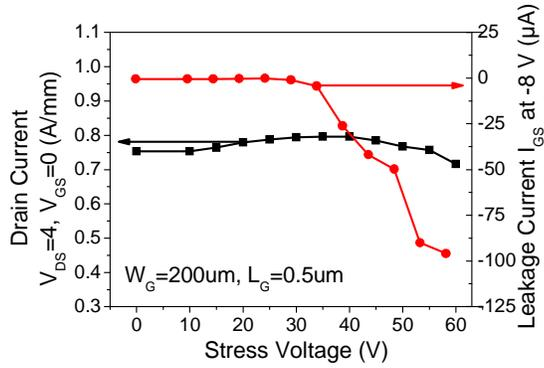
Fig. 1: variation of gate leakage and drain current for a HEMT submitted to a reverse-bias step stress experiment
