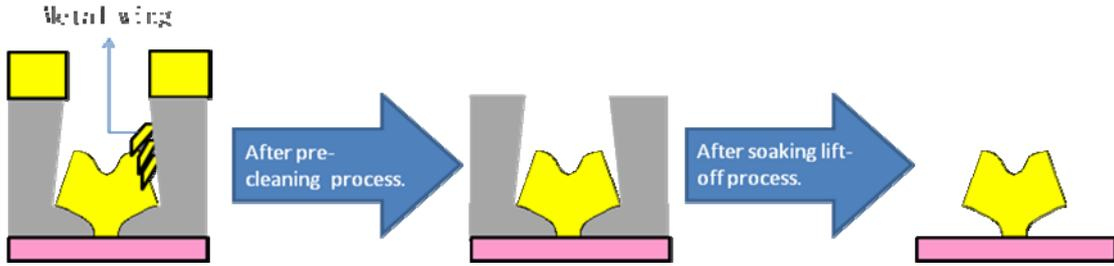
Figure 4, The concept of IPA spray type clean plus ACE soaking type clean
