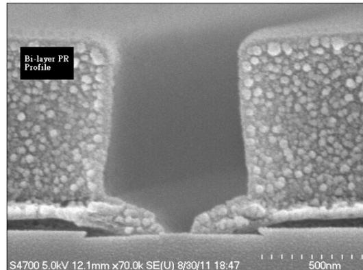
Figure 1, The bi-layer resistance profile of e-beam lithography technology.
