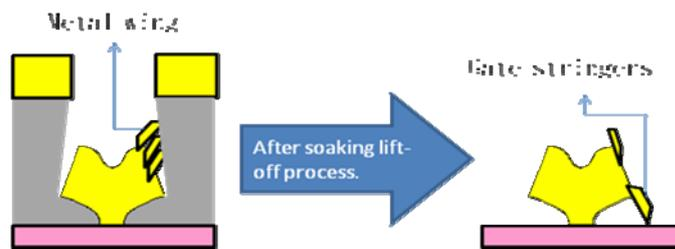
Figure 2, The mechanism of metal stringer.
