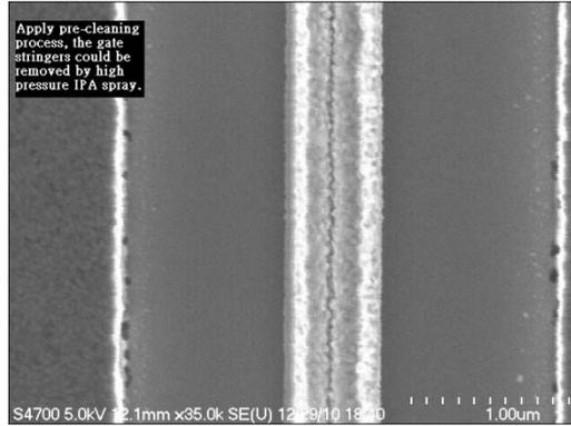
Figure 5, The SEM picture of the gate by using new lift-off process
