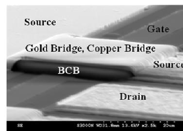
Fig. 1 The cross-sectional profile of the BCB-bridged AlGaIn/GaN power HEMTs.
