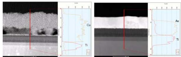
Fig. 5 The TEM images of Cu/Ti/GaN and Au/Ti/GaN interfaces after DC stress at high temperature.
