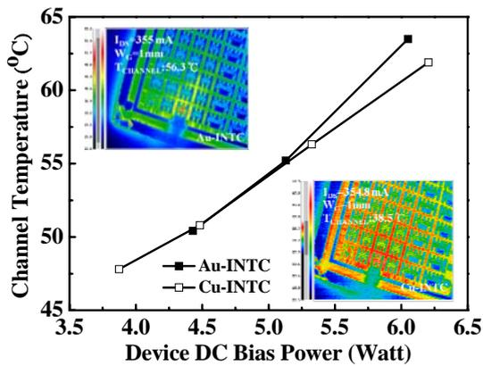
Fig. 2 Channel temperature performance of both devices versus various DC bias power values and IR images of AlGaIn/GaN power devices using Au-INTC and Cu-INTC designs.
