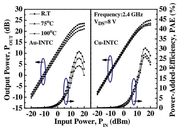
Fig. 4 Power performance of AlGaIn/GaN power HEMTs with Au-INTC and Cu-INTC versus temperatures at 2.4 GHz.
