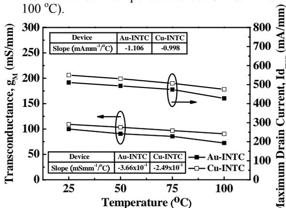
Fig. 3 The  $g_m$ ,  $I_{DS,max}$  temperature dependency curves for Au-INTC and Cu-INTC power HEMTs.
