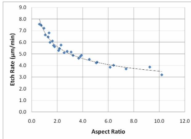
**Figure 2:** Time averaged etch rate as a function of aspect ratio for slot vias, from 20x25μm to 20x5μm slot vias.
