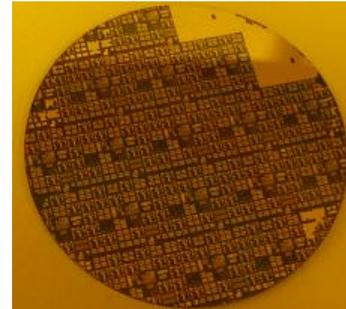
**Figure 2.** Picture of the 2-inch GaN on Diamond wafer
