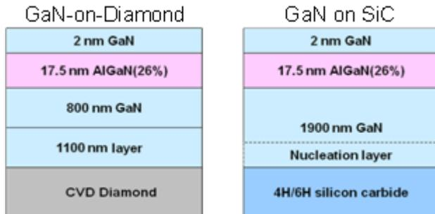
**Figure 1.** GaN epitaxial layers for diamond and SiC substrates were selected to be as close to each other as possible.
