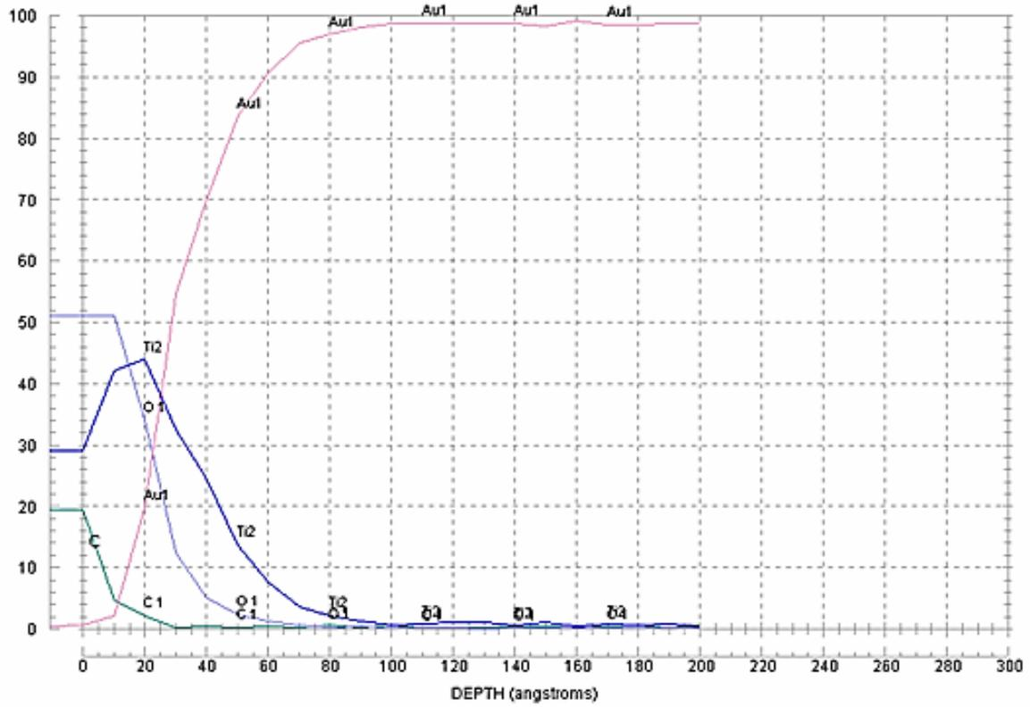
**Figure 1: Auger profile of bonding pad without any processing to remove Ti.**
