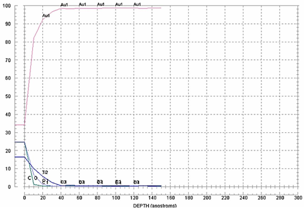
**Figure 3: Auger profile of bonding pad after SF6 dry etch**
