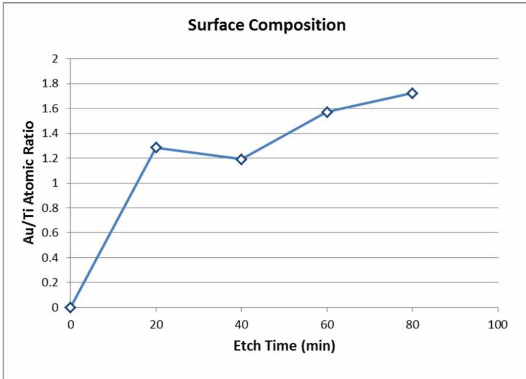
**Figure 4: Au/Ti surface composition ratio of bonding pad after concentrated acid wet etch**
