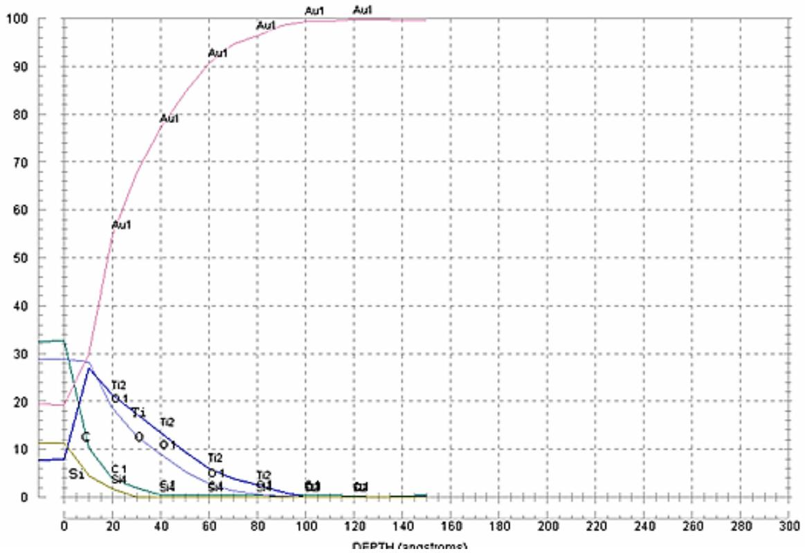
Figure 2: Auger profile of bonding pad after Ar sputter
