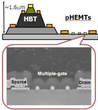
Fig1. SEM photograph of triple gate devices for rf-switch application
