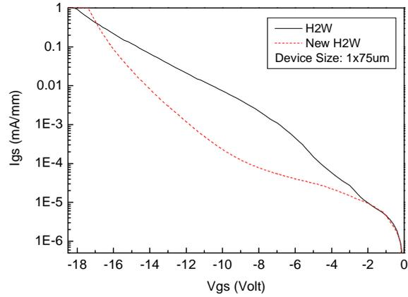
Fig3. Revised Schottky gate leakage characteristic of H2W.
