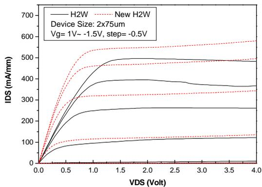
Fig2(b). The DC-IV characteristic comparison of H2W pHEMT devices
