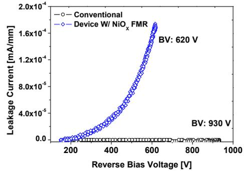
Fig. 4. Measured Breakdown voltage of the device with FMR
