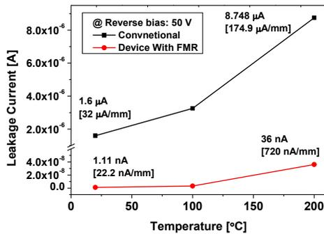
Fig. 2. Measured leakage current of the device with FMR
