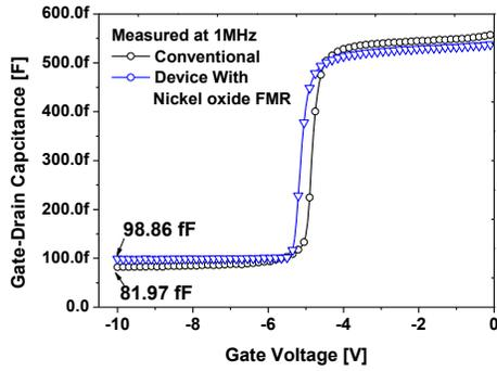
Fig. 1. Measured gate-drain capacitance of the device with FMR
