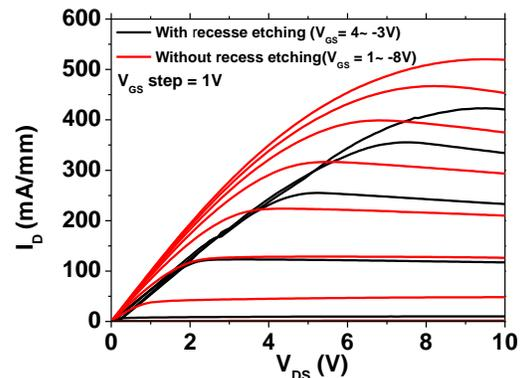
Figure 4. The measured  $I_D$ - $V_{DS}$  curves of HFETs with and without the gate-recessed etching.  $V_{th}$  for the recessed sample is 0.09 V and that for non-recessed sample is -6 V.
