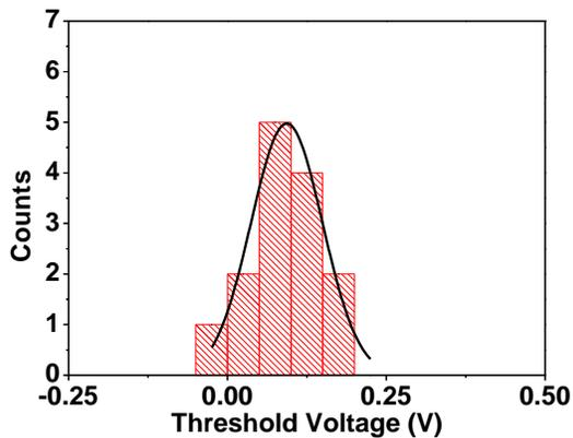
Figure 3. The histogram of measured threshold voltages of HFETs and the fitting of Gaussian distribution with mean of 0.09 V and standard deviation of 56 mV.
