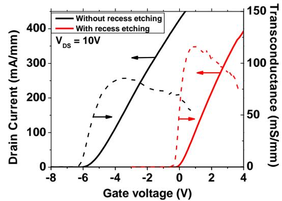
Figure 2. The measured  $I_D$ - $V_{GS}$  curves of HFETs with and without gate-recessed etching. The gate length of the device under study is 3  $\mu\text{m}$ .
