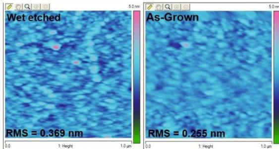
Figure 1. The surface morphology of the recessing etched surface (left) and the as-grown surface (right) measured by AFM.
