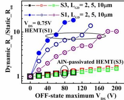
Fig. 3 Ratio of dynamic  $R_{on}$  and static  $R_{on}$  with varied OFF-state drain bias stress for S1 (without the RPP and passivation) and S3 (with the RPP and ALD-AlN passivation).
