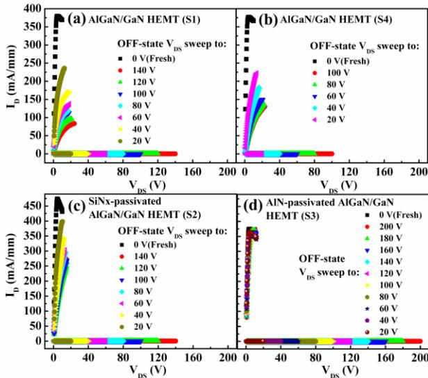
Fig. 2 Transient output characteristics of AlGaIn/GaN HEMTs with  $L_{GD} = 5$   $\mu$ m (a) without passivation and the RPP (S1), (b) without passivation but with the RPP (S4), (c) with  $SiN_x$  passivation (S2), and (d) with the RPP and ALD-AlN passivation (S3). The switching from OFF-state to ON-state is just once for each curve, and the switching time is  $\sim 70$  ns.
