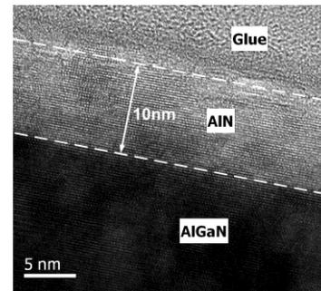
Fig. 1 HRTEM cross-section view of the interface between a 10 nm ALD-AlN and the AlGaN/GaN HEMT sample. Thicker AlN was used for observation purpose.
