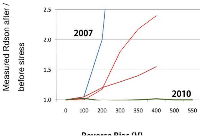
Fig 3: Measured Improvements in Dynamic  $R_{dsn}$  (=  $R_{on}$  after /  $R_{on}$  before stress)
