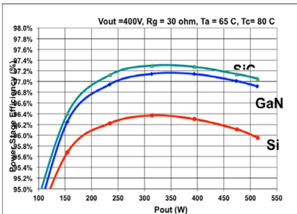
Figure 2: Measured power conversion efficiency for 150
