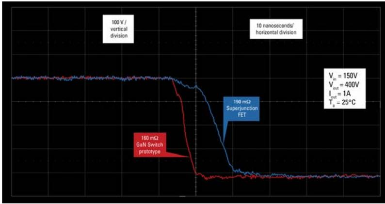
Figure1 : Turn-on waveform for 600 V
