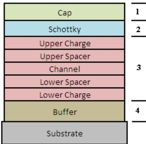
Figure 2: Schematic of a typical pHEMT structure. The five short duration layers from the lower charge to the upper charge (group 3) were found to be the contributors to the sheet resistance variation.
