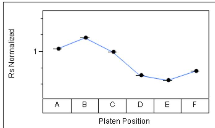
Figure 1: Sinusoidal sheet resistance pattern created by rotation effects on pHEMT structure at standard low RPM.
