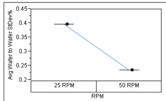
Figure 3: Over 40% improvement in wafer to wafer sheet resistance StDev% after increasing the rotation speed in the short duration layers to 50RPM.
