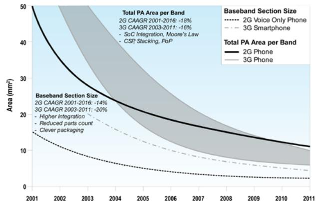
Fig. 3: Size reduction in baseband and PA sections
