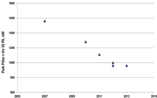
Fig. 4: Improvements in Peak Power Dissipation
