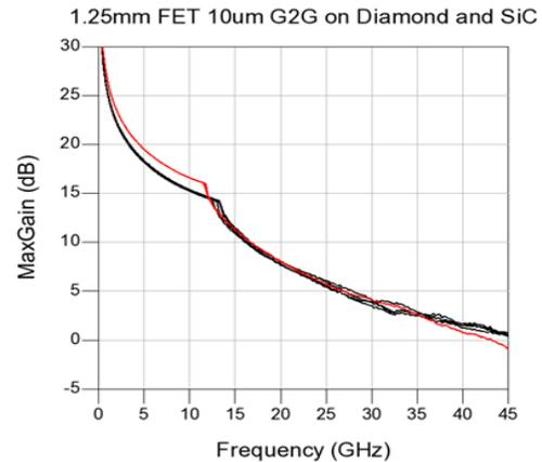
**Figure 3: Small-Signal MaxGain curves on 1.25mm FETs with 10um gate to gate spacing on GaN on Diamond (black) and GaN on SiC (red)**
