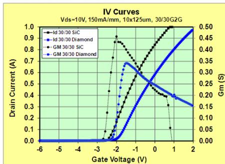
**Figure 2: Curves for a 1.25mm FET comparing performance on GaN on SiC and GaN on Diamond**
