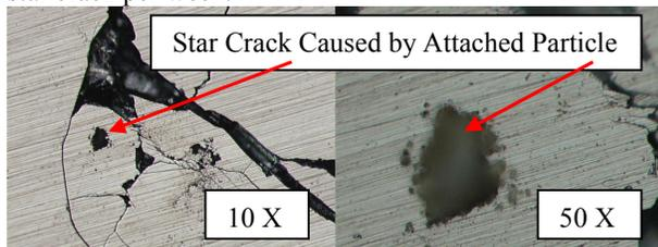
Figure 4: Star Crack Image
