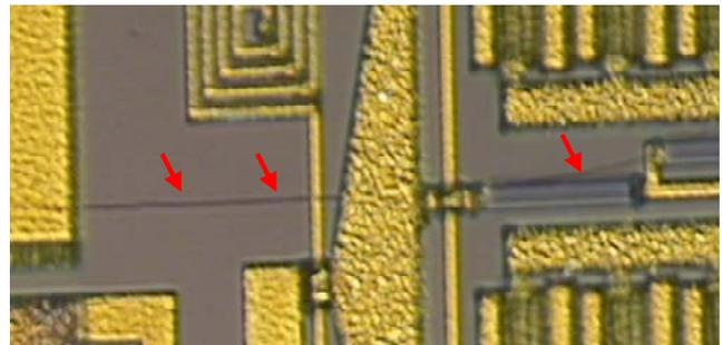
Figure 1: Example die fracture
