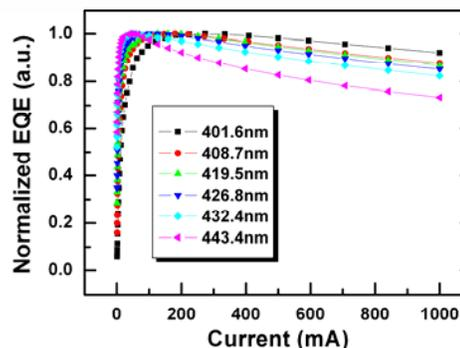
Fig. 3. Normalized external quantum efficiency with wavelength dependent LEDs as a function of forward current.
