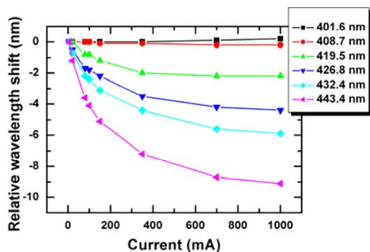
Fig. 2. Relative wavelength shift with wavelength dependent LEDs as a function of forward current.
