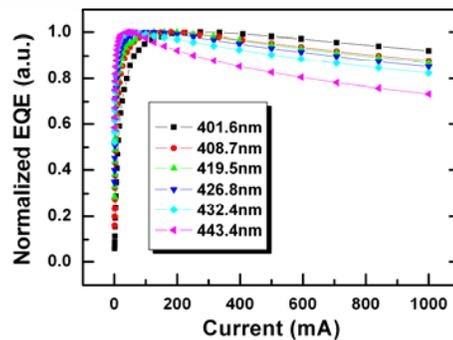
Fig.1. External quantum efficiency with wavelength dependent LEDs as a function of forward current.
