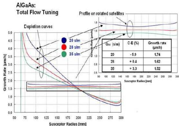
Figure 2: Modelling of growth rate depletion along susceptor radius for  $Al_{0.5}Ga_{0.5}As$  Layers
