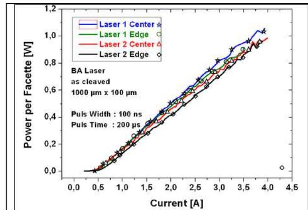
Figure 6: P(I) characteristics (left) of InGaAs BA laser devices with dimension 1000 μm x 100 μm.
