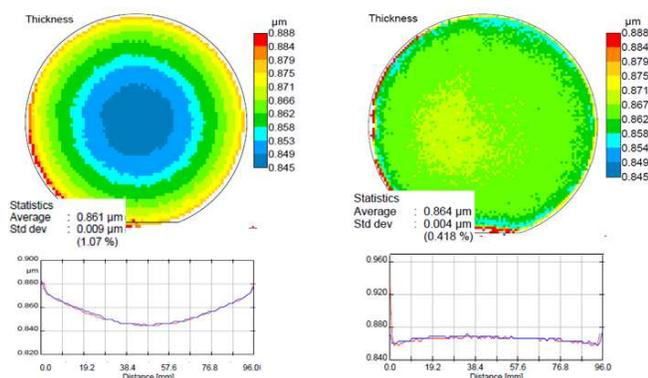
Figure 3: Thickness mappings for  $Al_{0.5}Ga_{0.5}As$  Layers using a total flow of 20 slm (left) and 28 slm (right)
