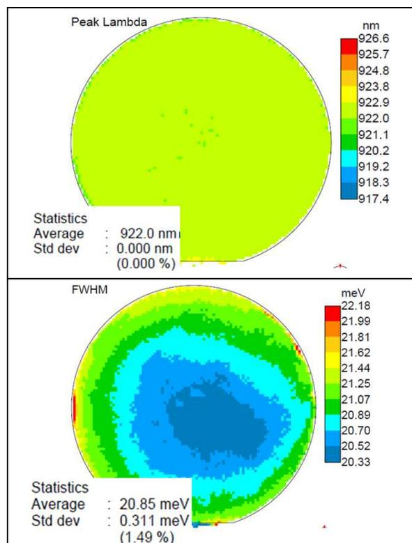
Fig. 4: Photoluminescence wavelength mapping of an InGaAs QW structure on exact orientated 4" GaAs substrate (Top) and respective FWHM mapping (Bottom)
