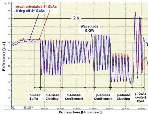
Figure 5: Reflectance Signal (952 nm Diode) during growth of an InGaAs laser structure grown on exact orientated and 6° off orientated substrate.
