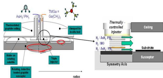
Figure 1: Schematic for flow-injection inside the reaction chamber separating group V and group III precursor materials providing additional flow-tuning.
