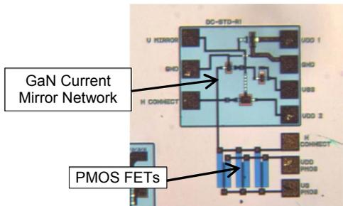
**Figure 4: Optical micrograph of Raytheon/MIT's monolithic heterogeneously integrated GaN HEMT+CMOS RF power amplifier circuit (adapted from [15]).**
