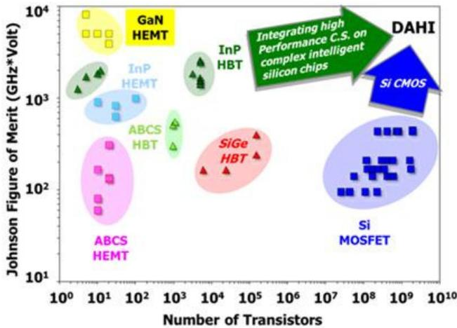
**Figure 1: Plot of Johnson Figure of Merit (product of transistor cutoff frequency and breakdown voltage) vs. Integration Complexity (number of transistors per circuit) classified by a variety of material and device technologies.**
