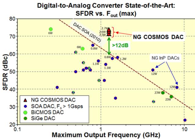
**Figure 3: Plot of SFDR vs. maximum output frequency of state-of-the-art DACs. Northrop Grumman (NG) COSMOS data points are shown in red.**
