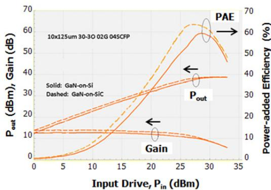
**Figure 5: Representative microwave measurements at 10GHz for the GaN HEMTs shown in Figure 4 (solid lines), as well as control samples fabricated on SiC substrates (dashed lines) (adapted from [15]).**
