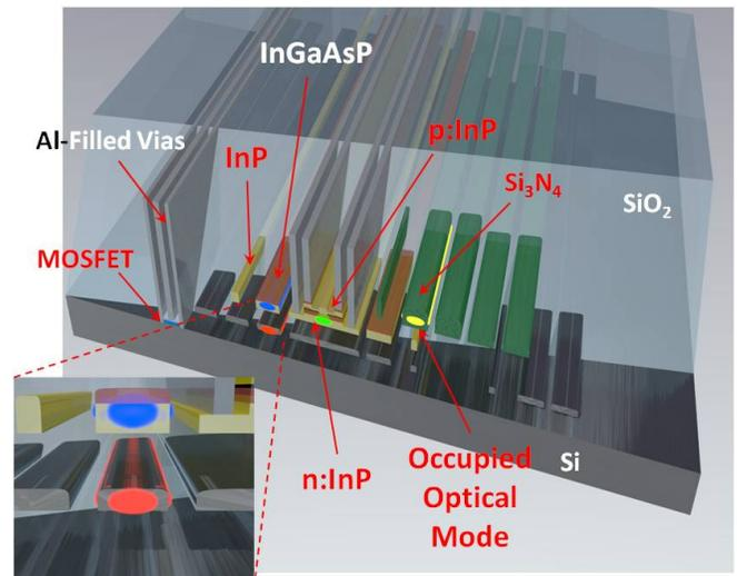
**Figure 6: Conceptual drawing of electronic-photonic heterogeneous integration platform to be developed in DAHI. Image courtesy of S. Radic, Univ. of California – San Diego.**
