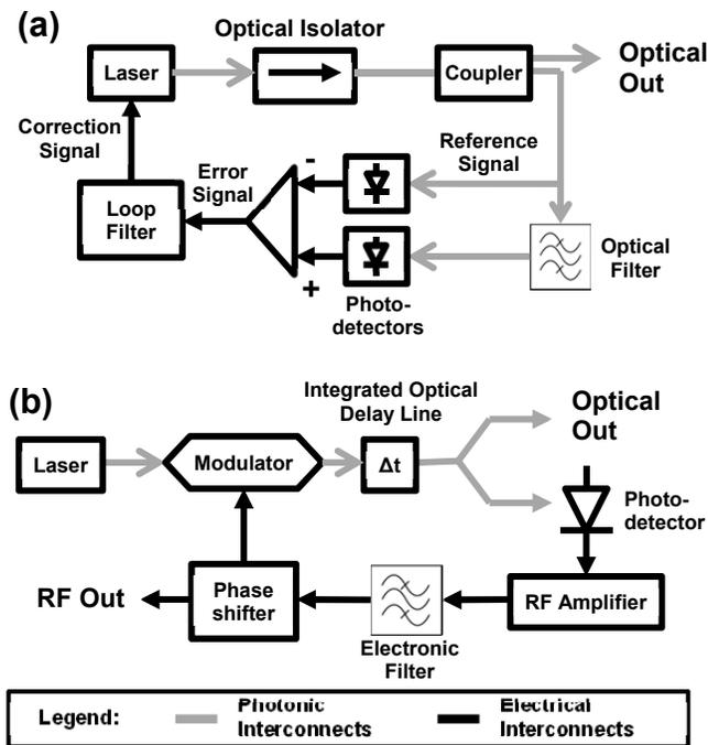
**Figure 7: Representative block diagrams of E-PHI demonstration microsystems, (a) frequency-stabilized laser source, and (b) RF opto-electronic signal source.**
