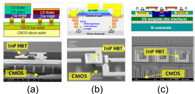
**Figure 2: Heterogeneous integration processes being pursued in the COSMOS program, (a) micrometer scale assembly, (b) epitaxial layer printing, and (c) monolithic epitaxial growth using a multi-layered lattice-engineered substrate.**
