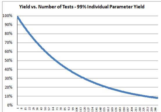
Fig 5: Overall Yield Curve vs. Number of Tests for 99% Exclusive Yield
