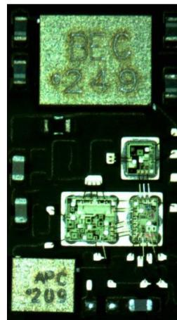
Fig 2: RFIC multi-chip module as assembled
