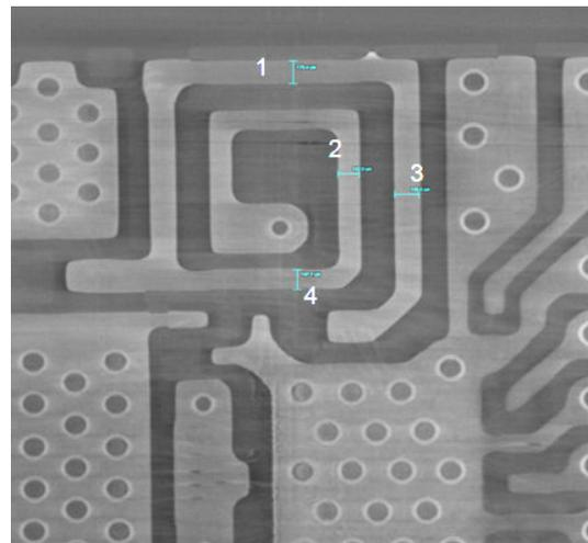
Fig 8: Laminate trace measurements
