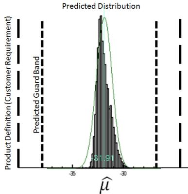
Fig 4: Illustration of Cpk Prediction
