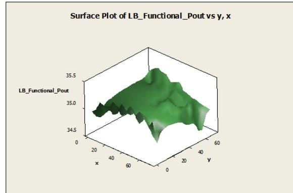
Fig 7: Power out vs. laminate panel location
