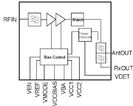
Fig 1: Typical RFIC module showing sub components
