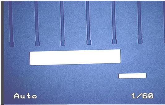
Figure 1b Halo defect was removed by another rinse in a clean dryer.
