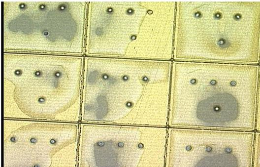
Figure 2a. Resist delamination from the plated gold on wafer backside.
