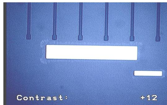
Figure 1a. Halo defect around resistor feature.
