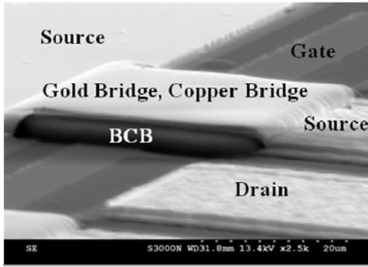
Fig. 1 The cross-sectional profile of the BCB-bridged AlGaIn/GaN power HEMTs.
