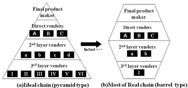
Fig.7 Types of supply chain. We found lots of barrel type in reality<sup>7)</sup>
