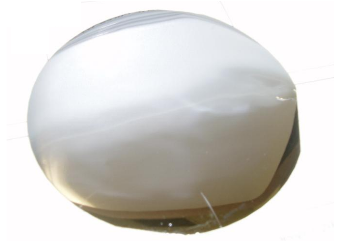
Figure 8: Four-inch-diameter ELO foil lifted off from an InP substrate.
